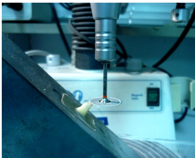
Figure 3.17 The fixed specimen subjected to a horizontal cut by using diamond disc attached the surveyor
