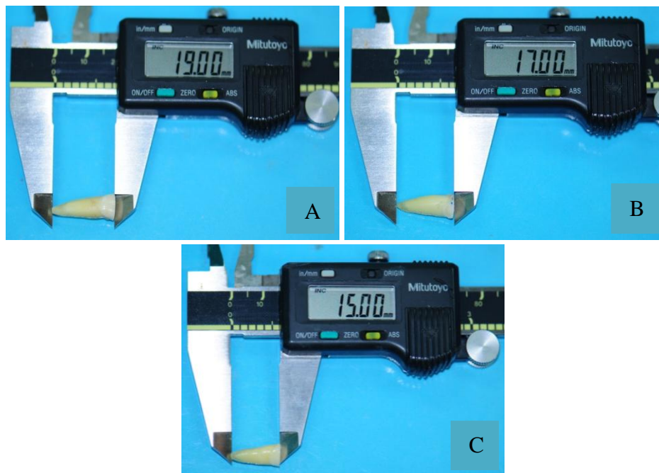
Figure 3.7 Specimen's lengths were assigned as: (a) 19 mm, (b) 17 mm and (c) 15 mm using digital caliper.
