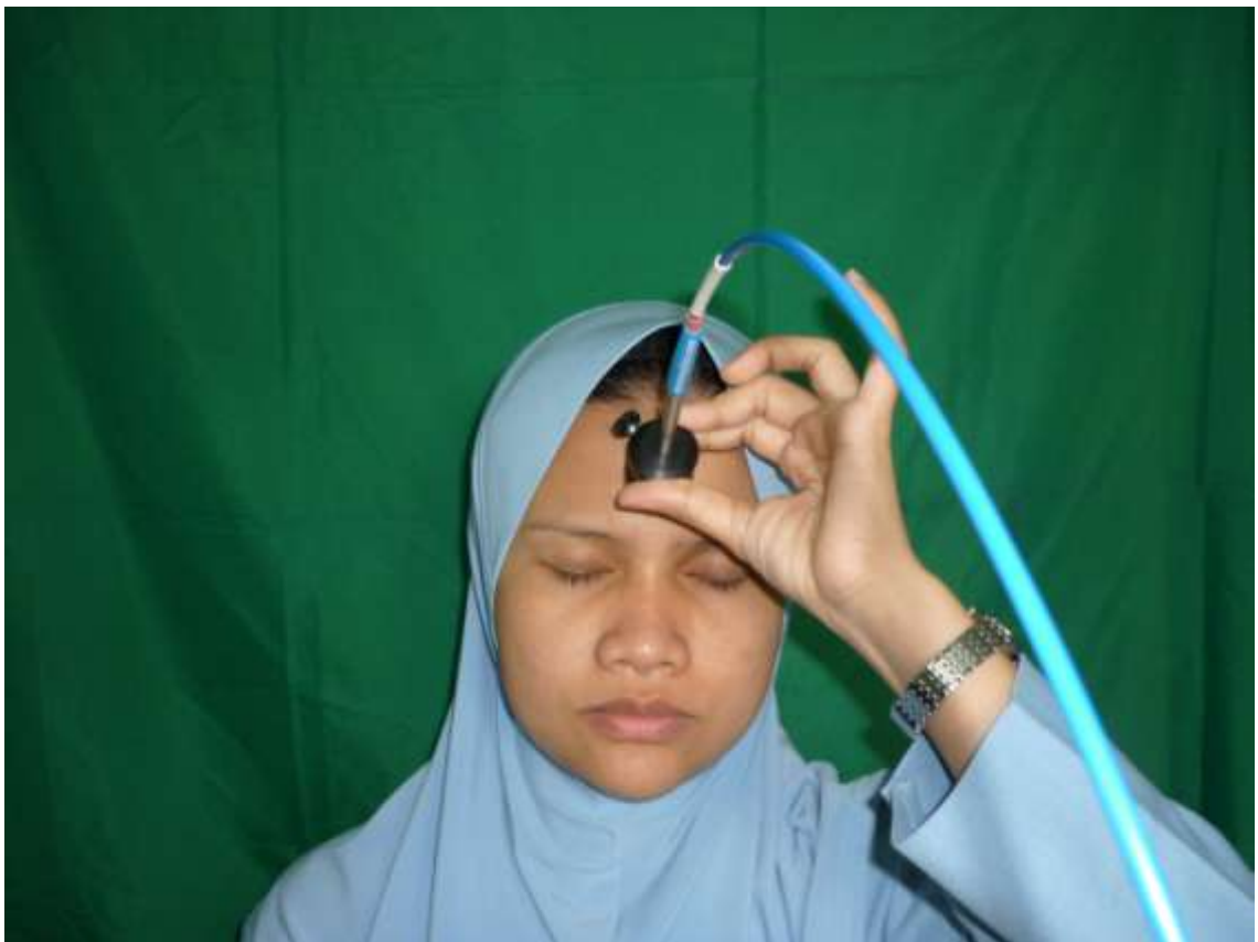
Figure 3.2 Spectrophotometer probe location on the forehead of the face when recording of skin tone was made.
