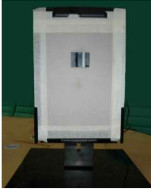
Figure 3.6 The scanner held vertically in the custom made jig with the cover removed.
