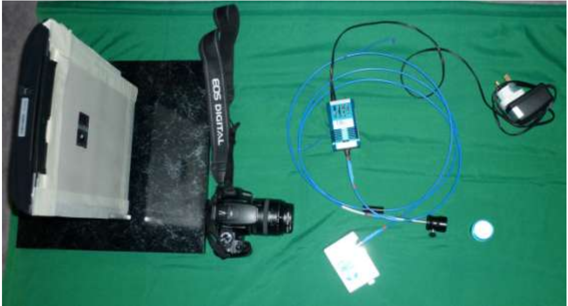
Figure 3.1 The spectrophotometer, digital camera and scanner used in the study.
