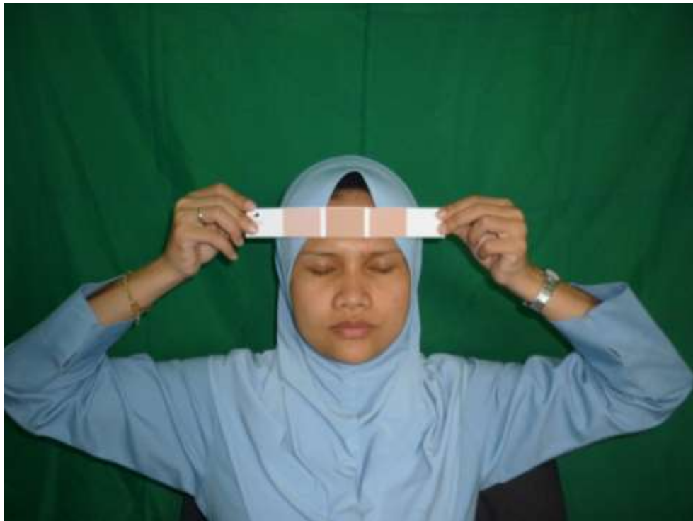
Figure 3.13 The printed skin tag was held closely to the forehead of the subject when colour matching was evaluated visually by assessors.
