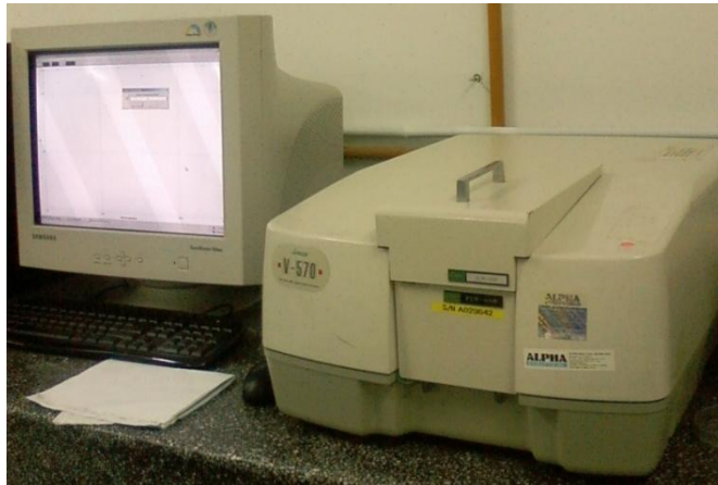
Figure 7.35: The set up of the “spectrophotometer” for measuring the solar optical properties of water.
