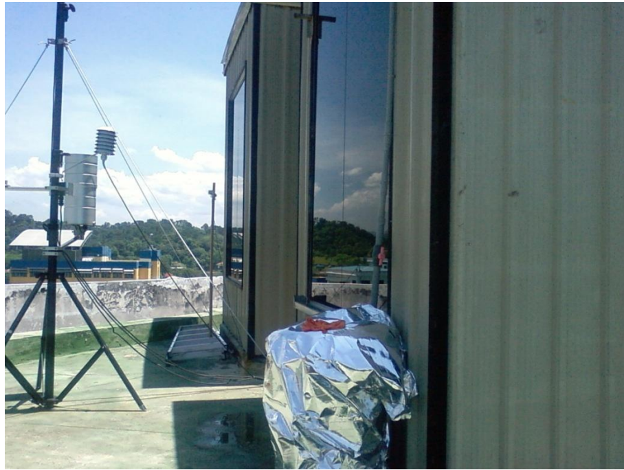
Figure 6.10: During experiments, the water reservoir was shaded by an aluminum foil
