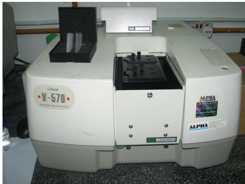
Figure 6.17: UV/VIS/NIR spectrophotometer to measure water spectrum
