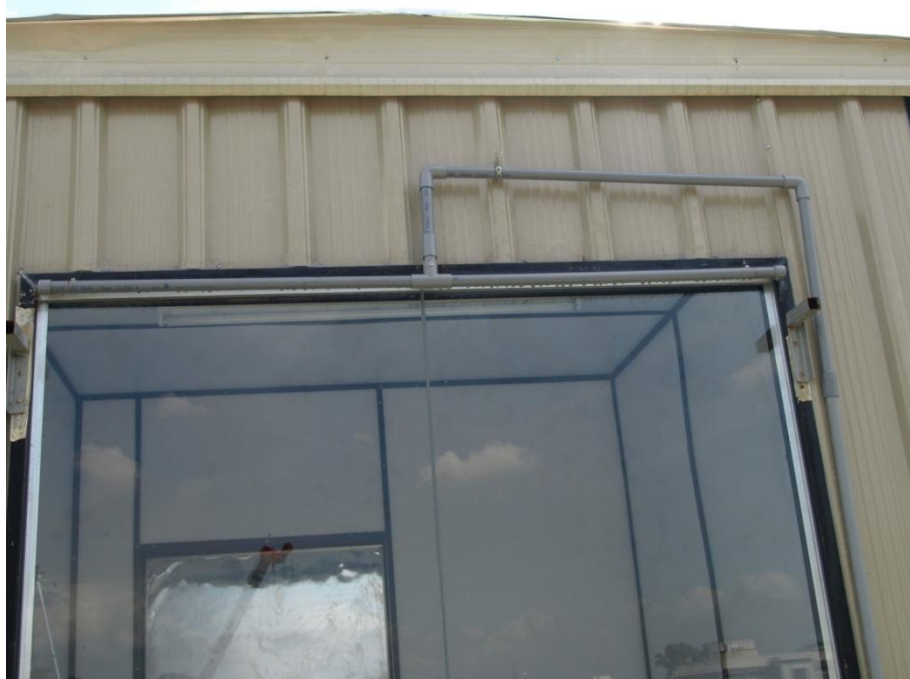
Figure 6.11: Feeding the water to the system comes through a t-junction with a pipe going right and left with both ends capped off.
