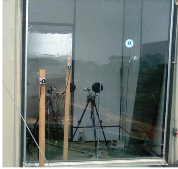
Figure 7.22: The view of the tested west facade showing the pyranometers that measured the internal/external vertical solar radiation of the CG façade.
