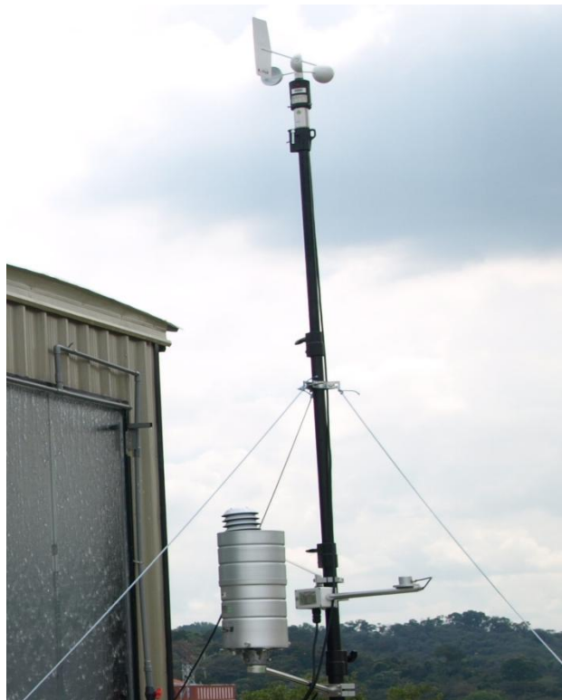
Figure 6.16: Set up of the weather station for measuring the outdoor experiment's variables
