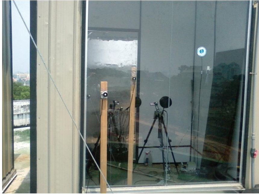
Figure 6.15: The vertical solar radiation monitoring sensors, which are attached to the wooden tripod.
