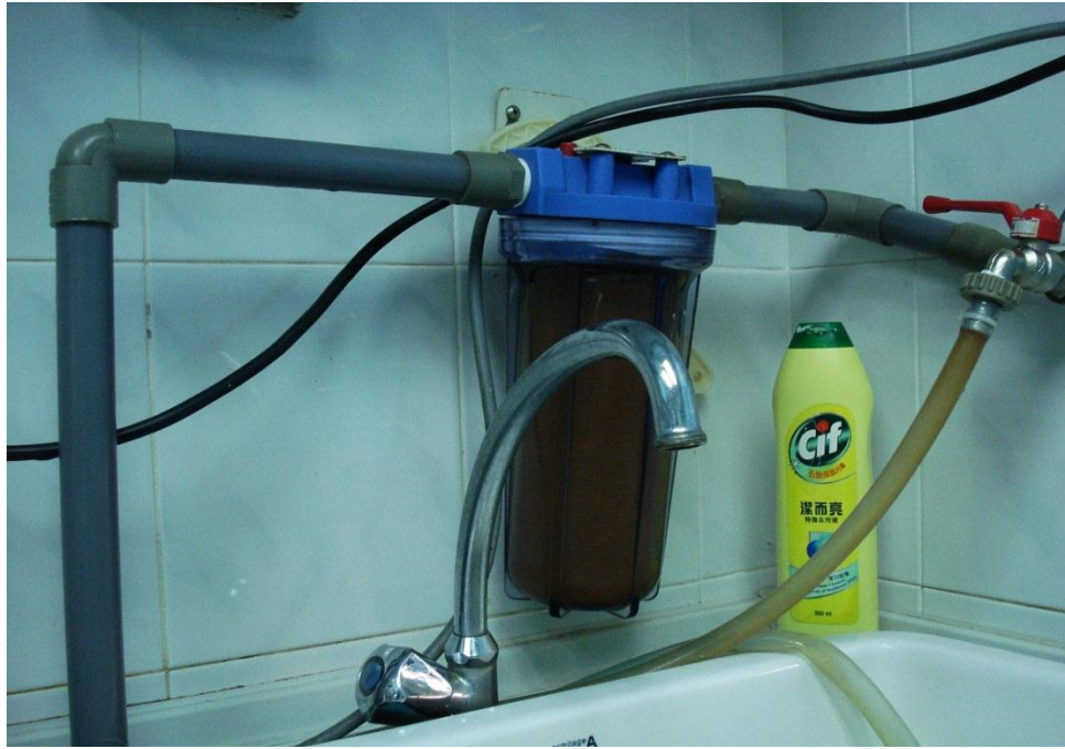
Figure 3.3: The filter unit used to filter municipal water prior to distillation.
