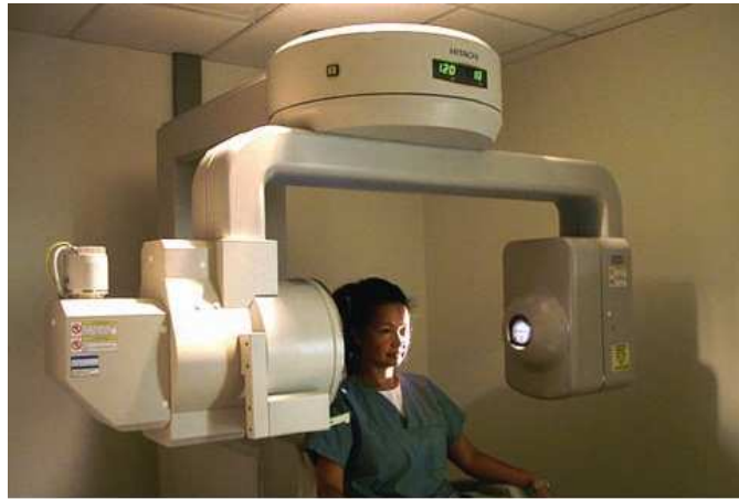
Figure 2.10: Cone beam computed tomography system showing the x-ray source (to the left of the model) and the receptor (Lam, 2007).
