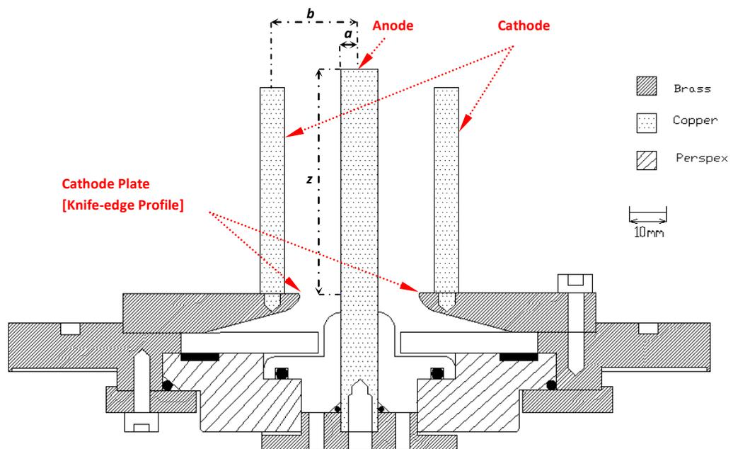
**Figure 2.1** The cross section of a plasma focus electrodes set.
