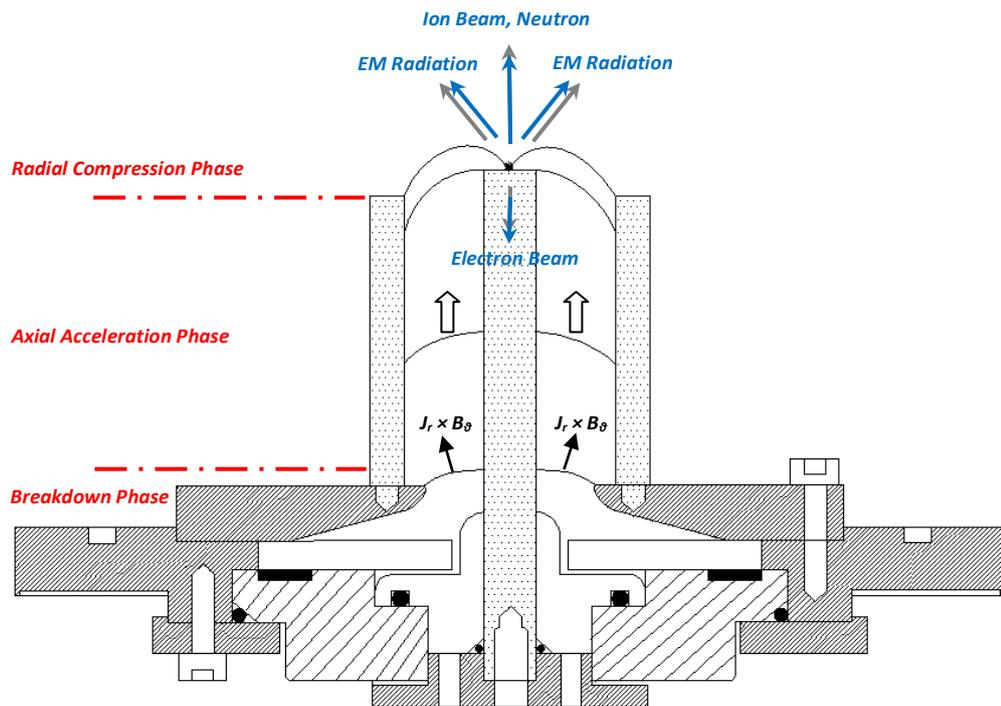
**Figure 2.2** The plasma focus tube. Current sheath in the breakdown phase, axial acceleration phase and radial compression phase is indicated at the respective position. Emission from the plasma pinch is also schematically indicated.
