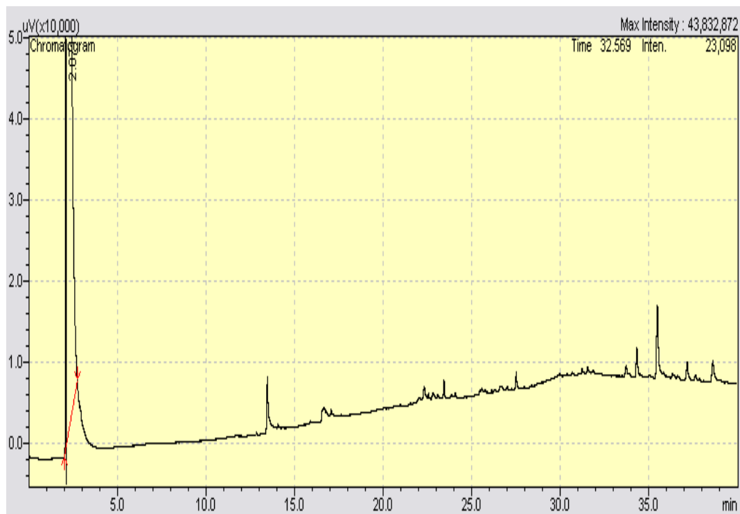
Appendix I (viii): GC-FID chromatogram of methanol crude extract from browning cells of suspension culture
