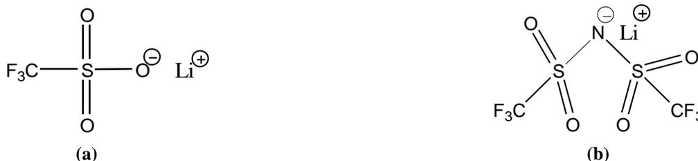
**Figure 2.5 Chemical structures of (a) lithium triflate and (b) lithium imide**
