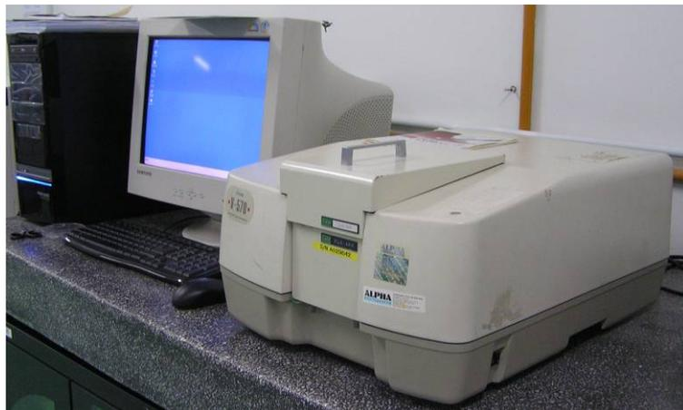
Figure 3.7: JascoV-570 UV-Vis-NIR spectrophotometer used for optical characterizations.
