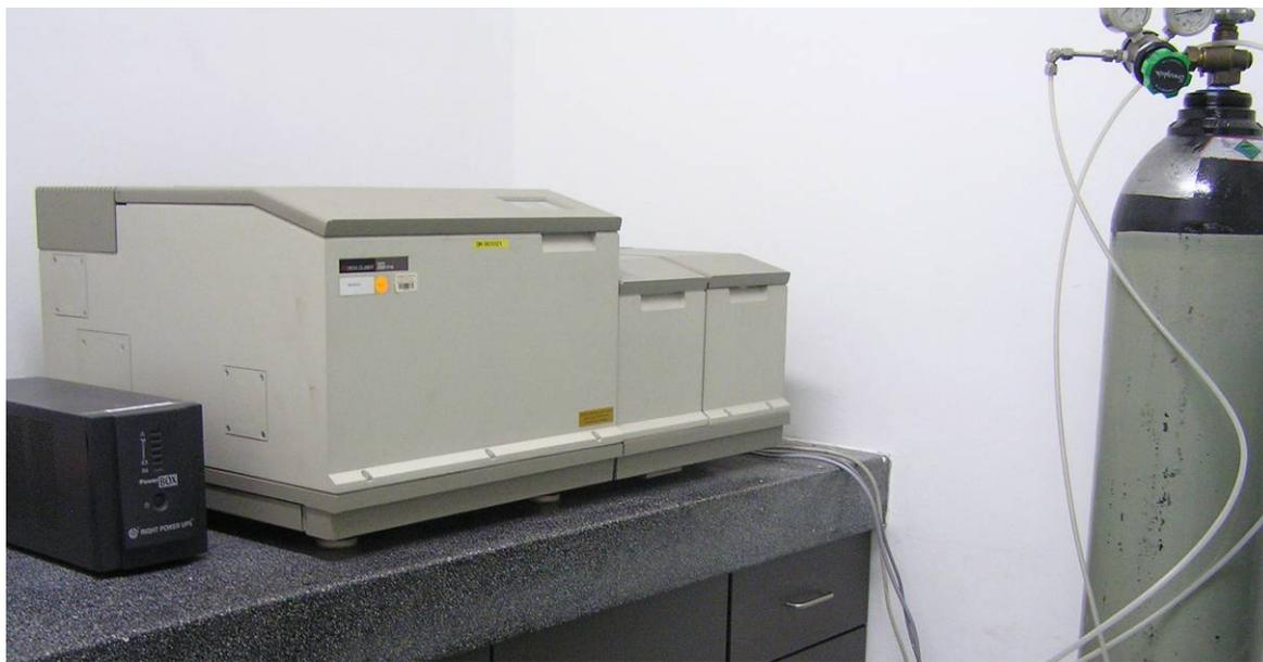
Figure 3.16: Perkin Elmer System 2000 FTIR used for chemical bonding studies.
