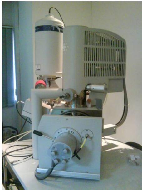
Figure 3.20: FEI Quanta 200 field emission scanning electron (FESEM) microscope used for surface and cross-sectional high-resolution imaging of carbon nitride films.
