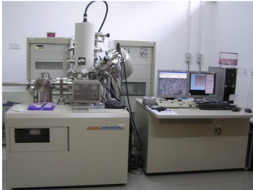
Figure 3.13: JEOL JAMP-9500F field emission Auger microprobe used for elemental composition measurements
