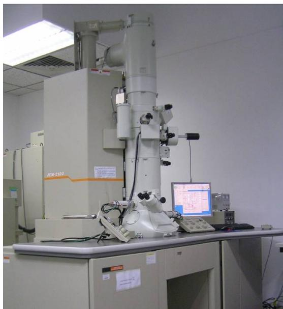
Figure 3.21: JEOL JEM-2100F high resolution transmission electron microscope used for high resolution imaging of individual nanostructured carbon nitride strands, energy dispersive x-ray (EDX) and selected area electron diffraction (SAED) analysis.
