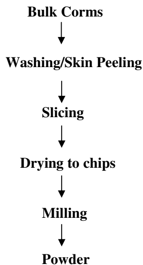
Figure 4.1: Steps involved in the preparation of powder samples from Amorphophallus spp.
