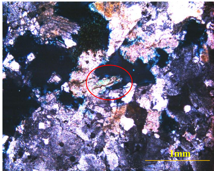
Plate 5.36 Muscovite (red circle) in pore space of Piring Hill rhyolite thin section.
