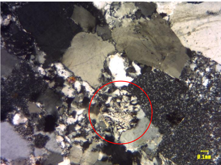
Plate 5.20 Thin section of sample HL2 showing spherulitic texture of rhyolitic igneous rock fragment (Circle) that similar to the rhyolite rock in Piring Hill, Tatau.
