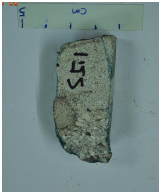
Fig. 5.8 Hand specimen of Ransi Member graded pebbly sandstone from facies F2, locality L2, Tutong Hill.
