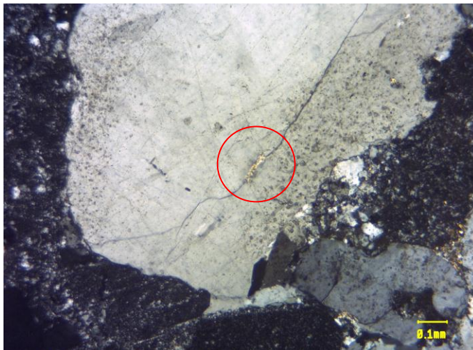
Plate 5.10 Thin section of TT3 showing quartz overgrowth and pseudomatrix (in cycle) within the quartz grain at locality L4, Tatau Hill.
