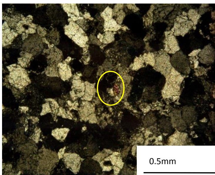
Plate 5.18 Thin section of sample HL7 showing mica inclusion (in circle) within quartz grains for source provenance.
