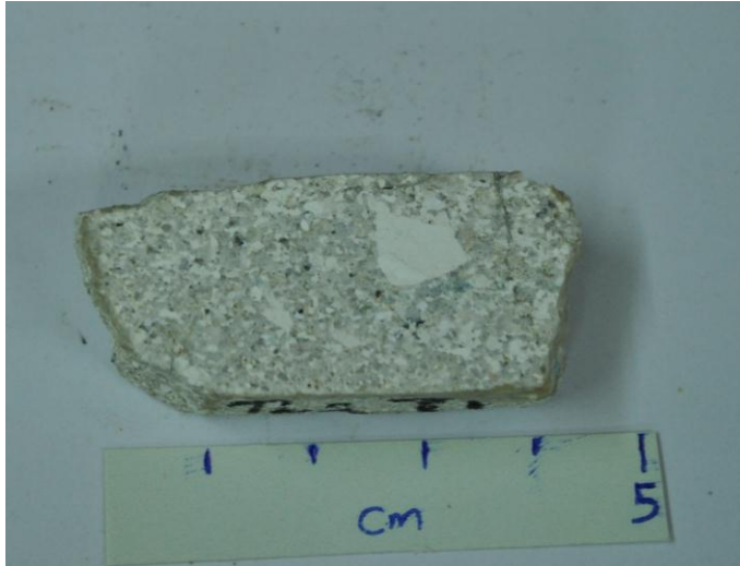
Fig. 5.15 Hand specimen of quartz rich pebbly sandstone from TT2 at the lower section of Tatau Hill, locality L4.
