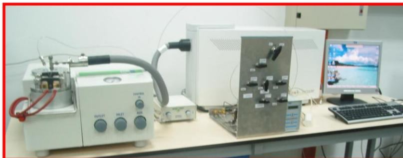
Figure 3.14: Differential Scanning Calorimeter for determination of melting points, phase change temperatures and chemical reaction temperature
