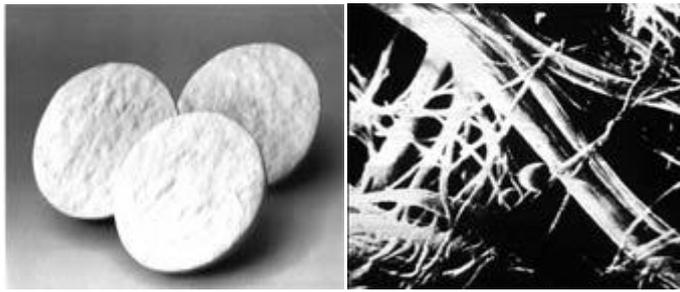
Figure 3.5. Glass fibre for sample filtration.
