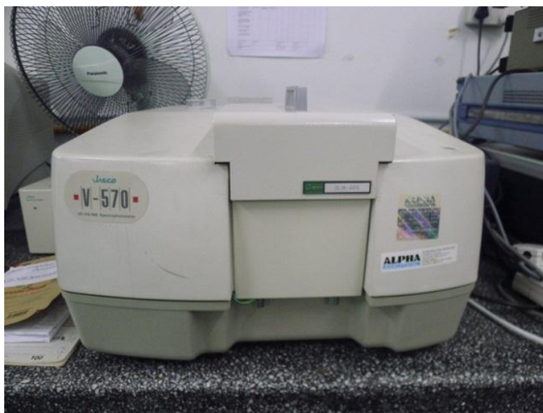
Figure 3.19 Photograph depicting the UV-VIS/NIR Spectrometer (model Jasco 570) that have been used to investigate the absorption properties.
