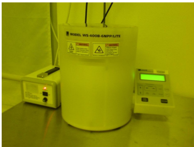
Figure 3.6 Photograph depicting the spin coater used in this research. The spin speed and time are set in the program provided by this machine
