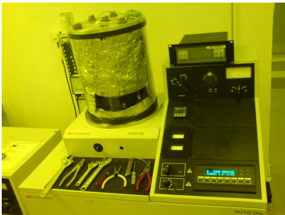
Figure 3.10 Photograph depicting the thermal evaporator (EDWARDS 306) used in this research
