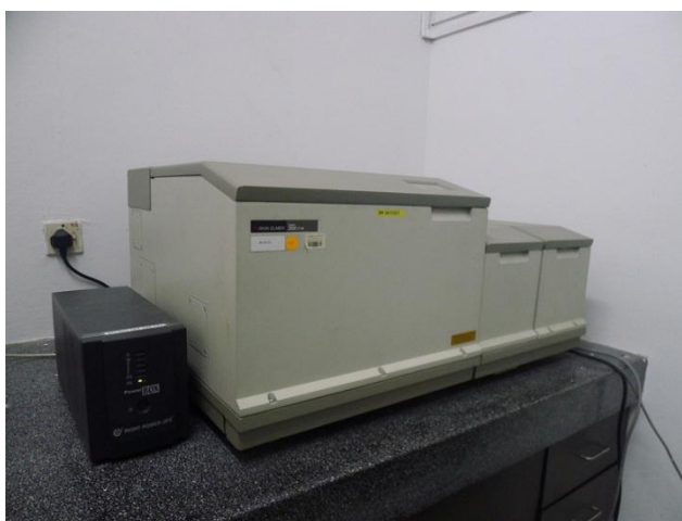
Figure 3.15 Photograph depicting the Perkin-Elmer System 2000 Fourier transforms infrared (FTIR) spectrometer that has been used to examining the FTIR spectra of the films
