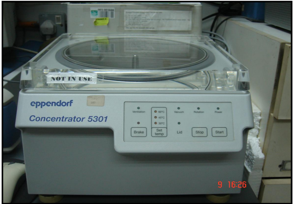
Figure 3.2.1c: Vacuum-concentrator used for concentrating the larval extract and removing methanol
