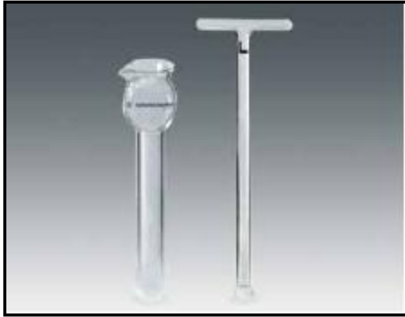
Figure 3.2.1a: 15-ml glass Dounce homogenizer used to homogenize L. cuprina late second-instar larvae
