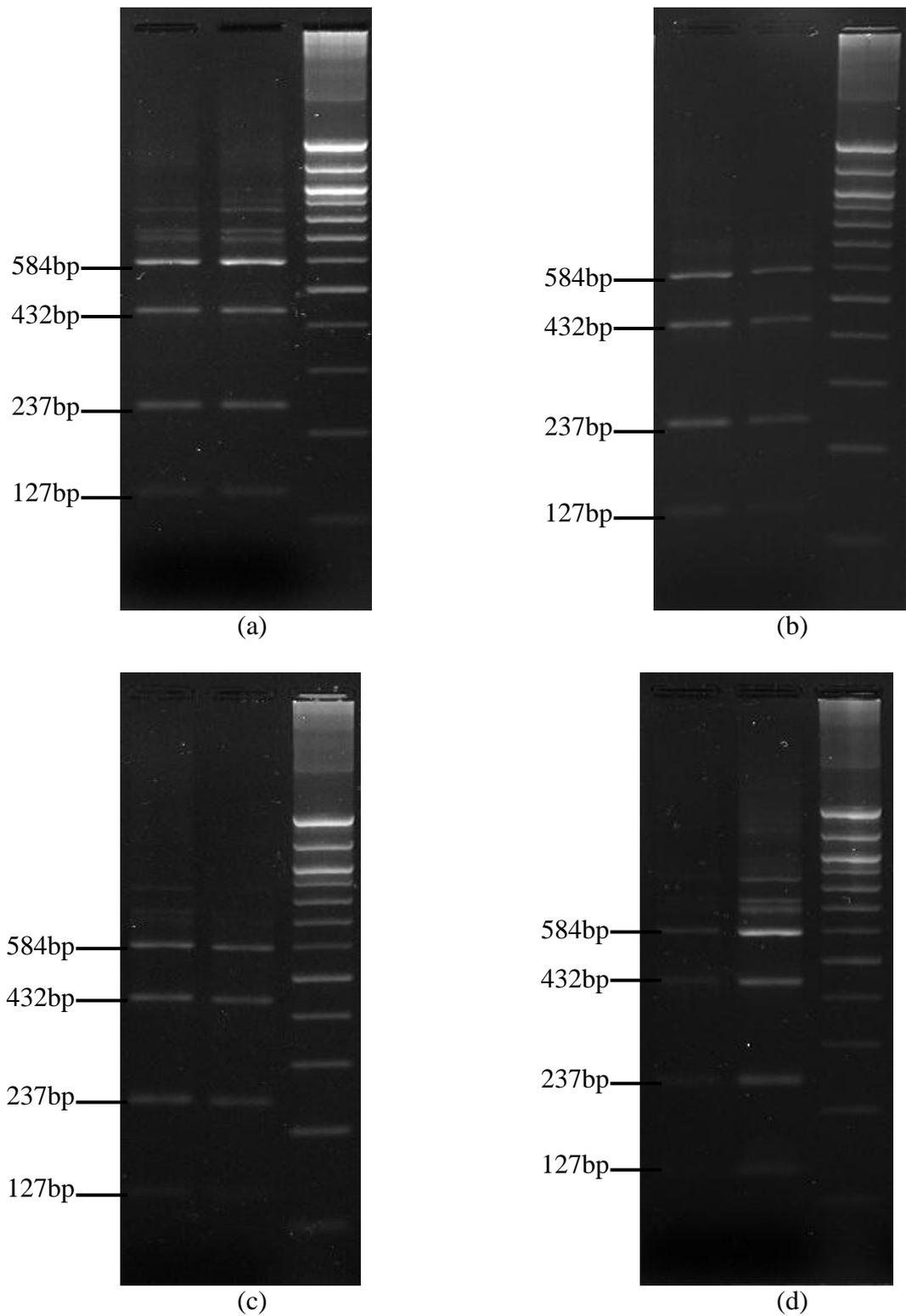
**Figure 6.9:** Identical RFLP profiles of COI digested with restriction endonuclease, *SspI* for (a) *L. dux*, (b) *L. saprianovae*, (c) *S. crinita* and (d) *S. inextricata*.
