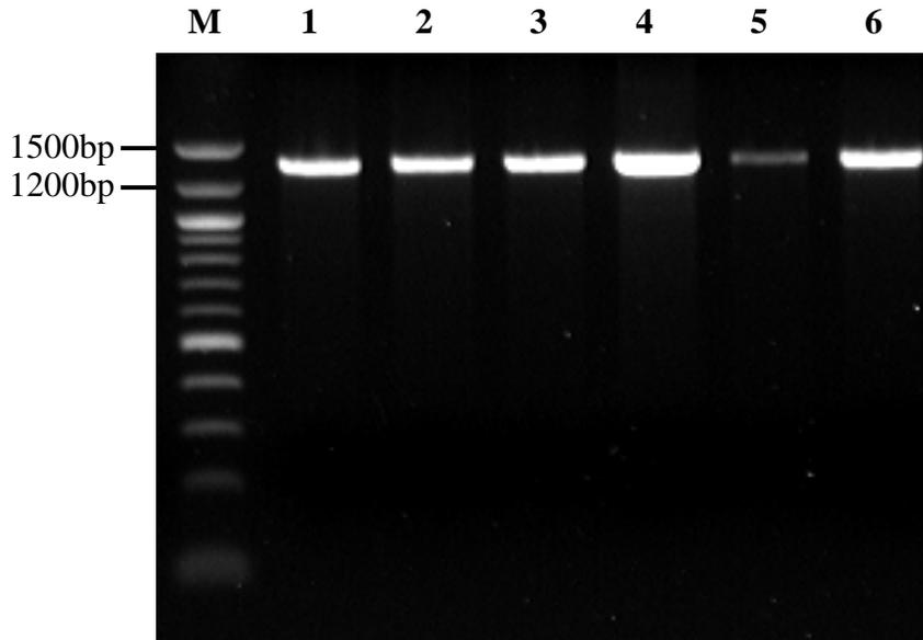
**Figure 5.16:** Purified PCR product of primer set C1-J-2495 and TK-N-3775 (~1324bp) after gel extraction. Lanes: M, molecular weight marker of 100bp DNA Ladder (New England Biolabs, UK) and 1-6, purified PCR products of species of Calliphoridae.
