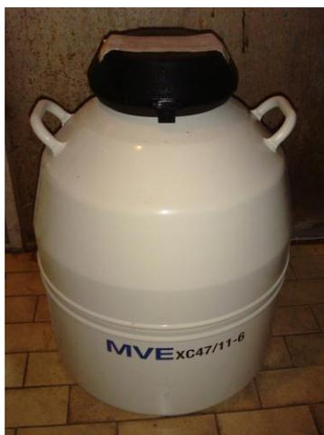
**Figure 2.11:** *Liquid Nitrogen Freezer (MVE).* Narrow-necked freezer with storage on canes in canisters at  $-196^{\circ}\text{C}$ .
