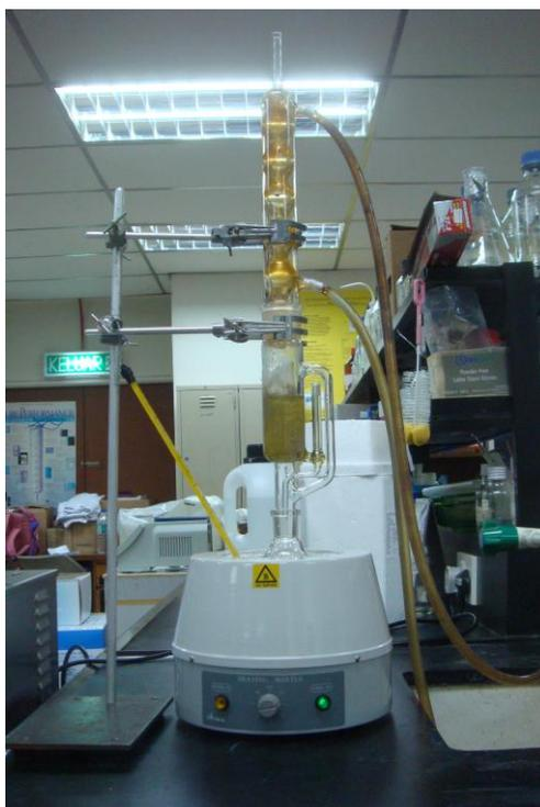
**Figure 2.20:** Conventional Soxhlet extractor system
