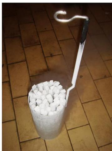
**Figure 2.13:** *Canes in Canister.* Cryovials are clipped onto aluminum cane, placed in the canister, and stored in the liquid nitrogen tank at  $-196^{\circ}\text{C}$ .
