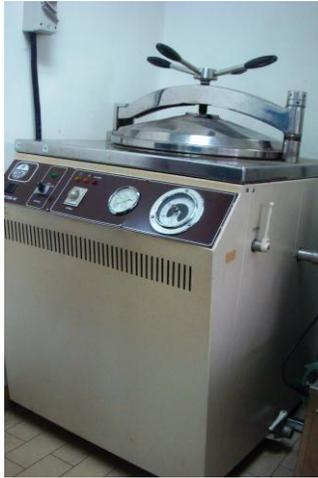
**Figure 2.3: Autoclave.** Heat-stable liquids such as distilled water and phosphate buffer saline used for cell culture works are sterilized by autoclaving.
