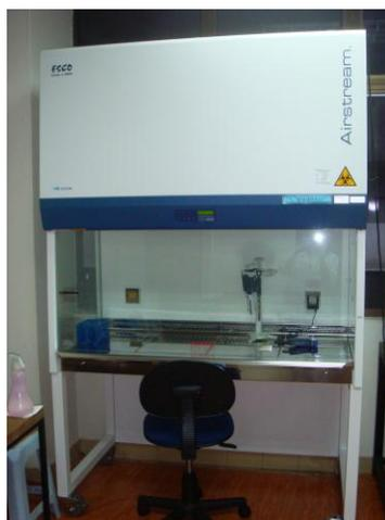
**Figure 2.6: Escco Class II Biohazard Cabinet.** A Class II biohazard cabinet is used to provide aseptic conditions for cell culture works in the laboratory.
