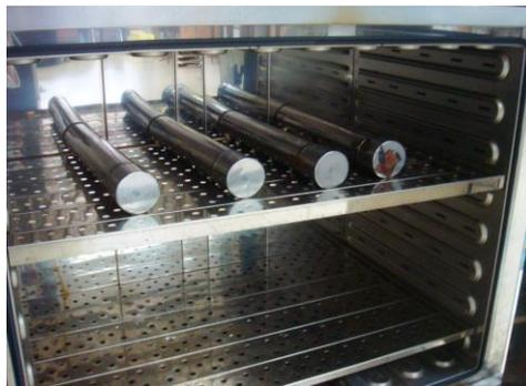
**Figure 2.2:** Pipette canisters were placed with spaces between to allow circulation of hot air in the sterilizing oven.
