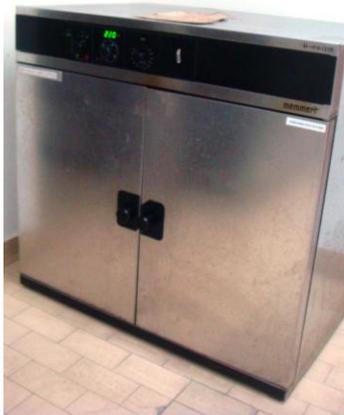
**Figure 2.1: *Sterilizing Oven.*** Dry heat sterilization of pipettes is carried out at 180°C for 2 hours.
