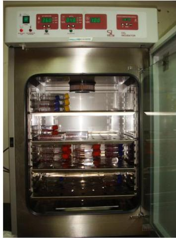
**Figure 2.10:  $CO_2$  incubator.**  $CO_2$  incubator (Shel Lab) with door open showing cell culture flasks and multi-well plates.
