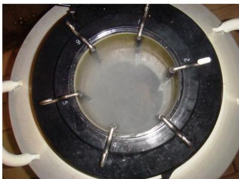
**Figure 2.12:** *Interior of Liquid Nitrogen Freezer.* Six canisters were positioned under shoulder of the freezer.
