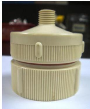
**Figure 2.4: Reusable filter.** Polypropylene, in line, Luer fitting or known as swinnex.
