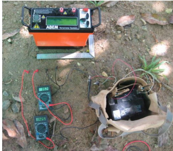
Figure 3.3. Measurement set up for Terrameter SAS4000 and standard device.
