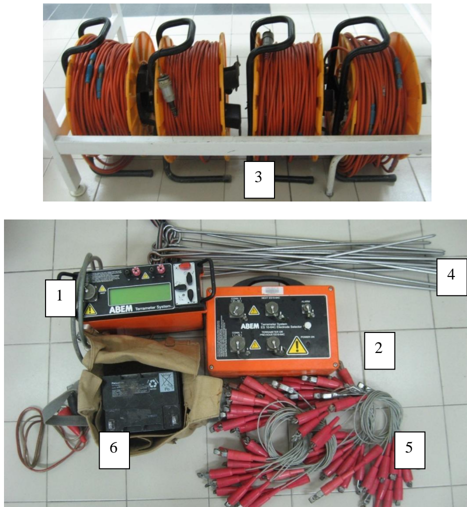
Figure 3.2. ABEM Terrameter SAS4000 and its accessories. 1) Resistivity meter, 2) Box of current selector, 3) Multiconductor cables, 4) Electrodes, 5) Connector, 6) Current source
