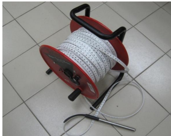
Figure 3.16. Deep meter for water level equipment.
