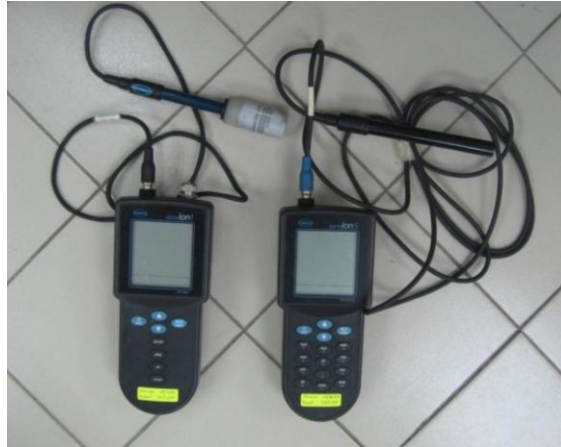
Figure 3.15. Equipment used in order to attain in-situ parameters: pH meter (left), and Conductivity-TDS-Salinity-Temperature meter (right).
