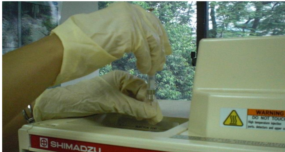
Plate 3.7: Injection of gas sample to GC
