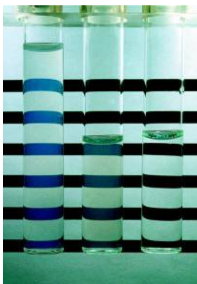
Figure 3.2: Comparison of McFarland 0.5 with inoculum suspension. From left to right, the tubes are the McFarland 0.5 standard and bacterial suspensions
