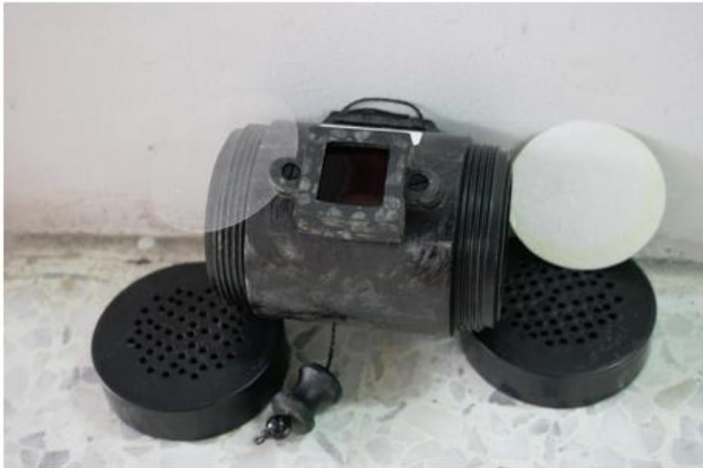
Figure 3.3: SSNTDs applied inside a canister dosimeter, the ‘twin radon-thoron cup dosimeter’
