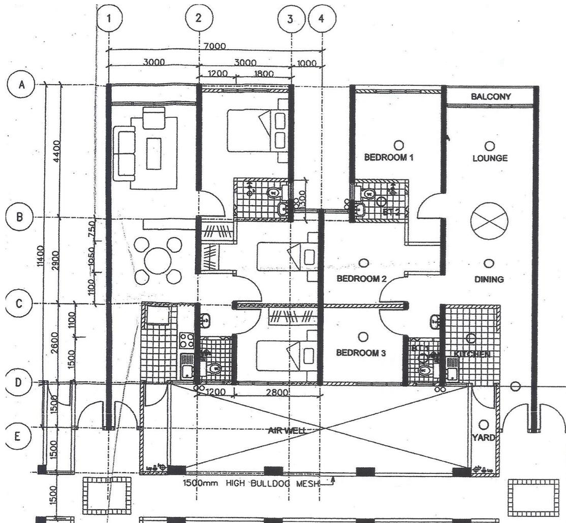
Figure 3.4 Internal layout plan of two neighbouring units (“BEDROOM 2” and “BEDROOM 3” sharing a common apartment building wall)
