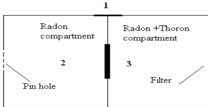
Figure 3.5 Twin radon-thoron dosimeter system
