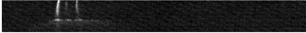
Figure 4.1: Image of the single negative current pulse in the 5 mm gap DBD captured by ICCD camera with gate width of 500 \mu s. Three synchronous breakdowns were observed in a single negative discharge current pulse.
