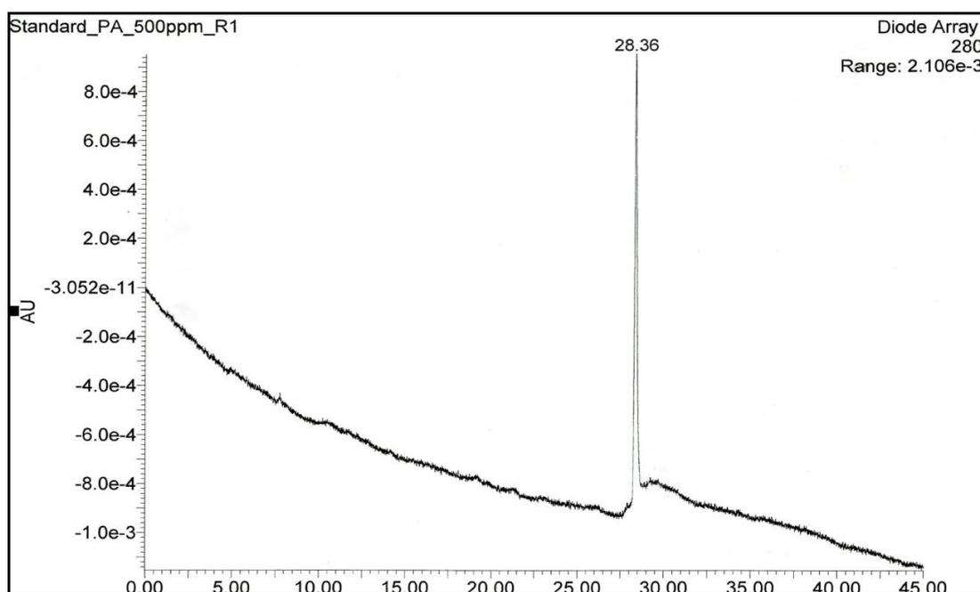
**Figure 3.17** : HPLC chromatogram of Phorbol 12-myristate 13-acetate
