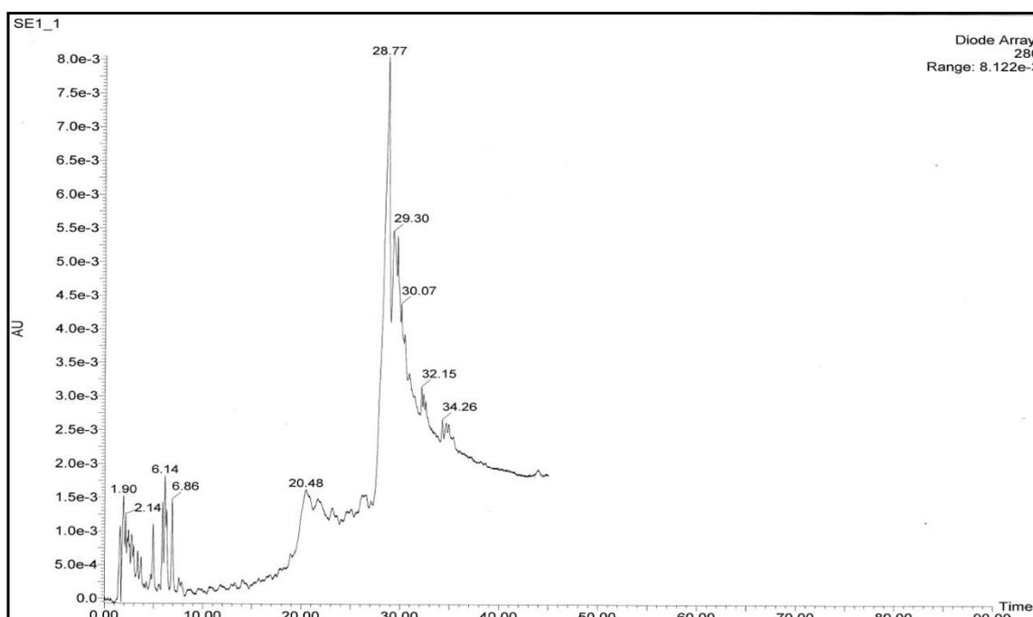
**Figure 3.18 :** HPLC chromatogram of experiment S1
