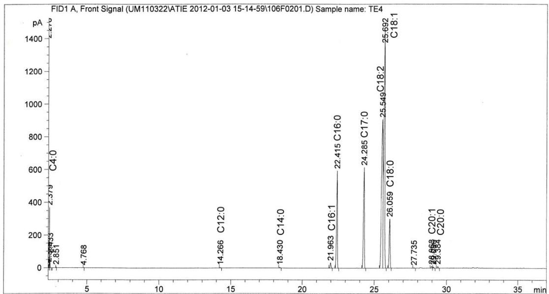
Figure 3.25 : GC chromatogram of experiment TE4 for ester content determination
