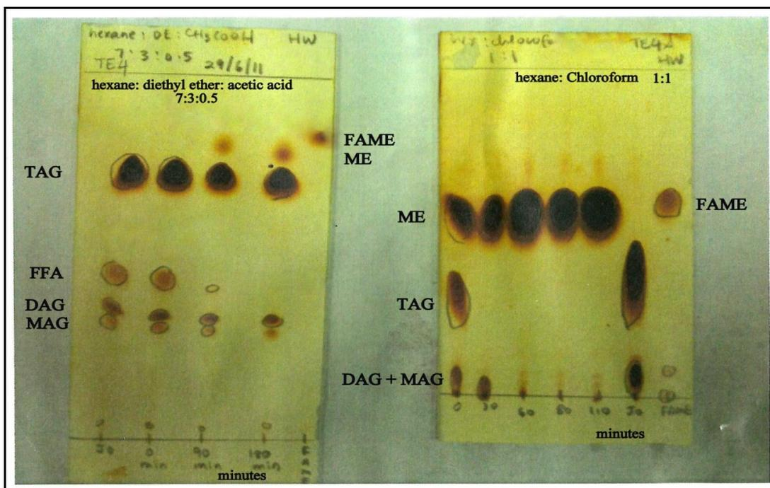
**Figure 3.12 :** Thin-layer chromatography of direct esterification and transesterification reaction
