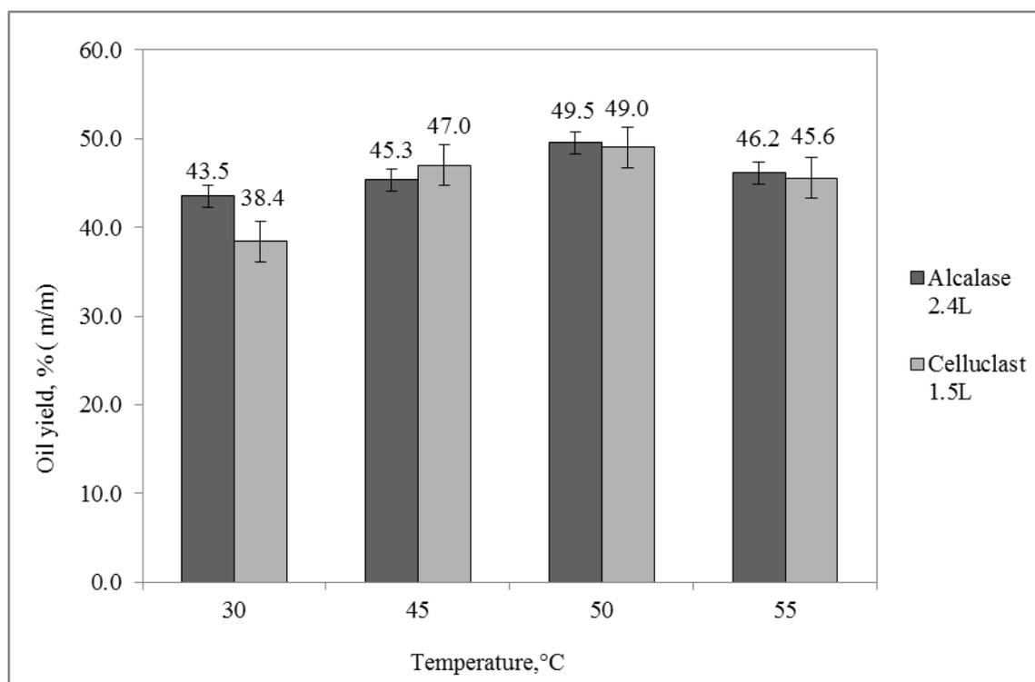
**Figure 3.6 :** Effect of varying incubation temperature in EAAOE
