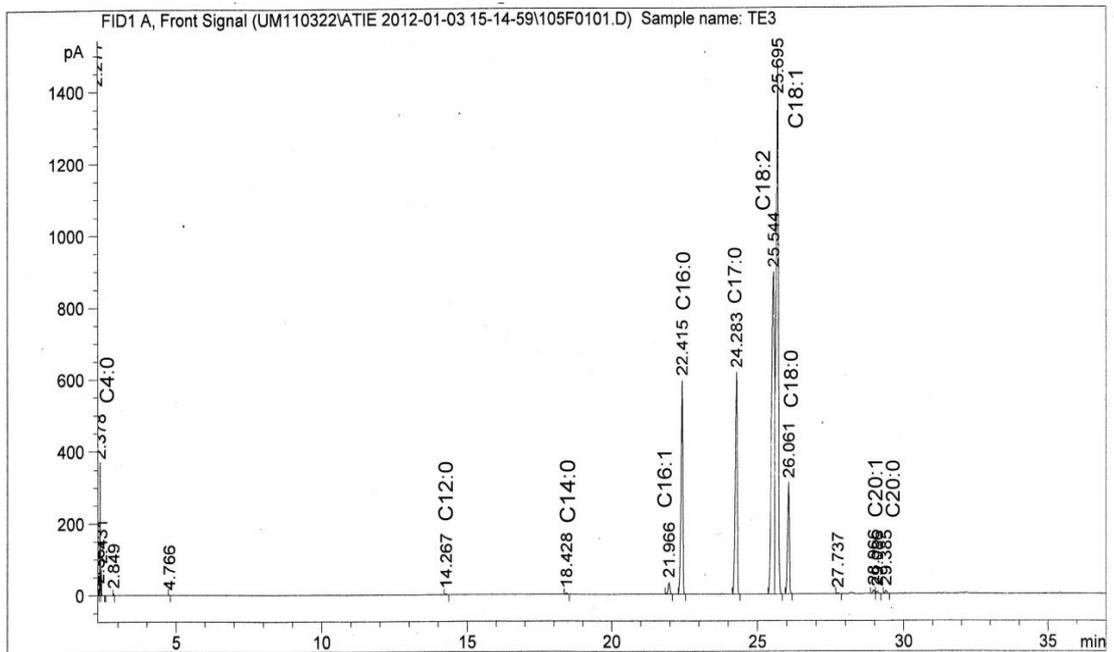
Figure 3.24 : GC chromatogram of experiment TE3 for ester content determination
