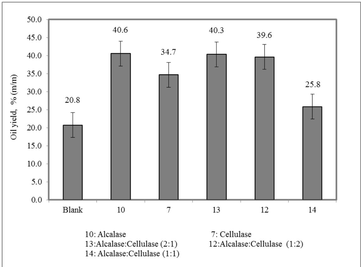
**Figure 3.1** : Comparison of percentage (%) on oil yield by singular and combination enzymatic extractions
