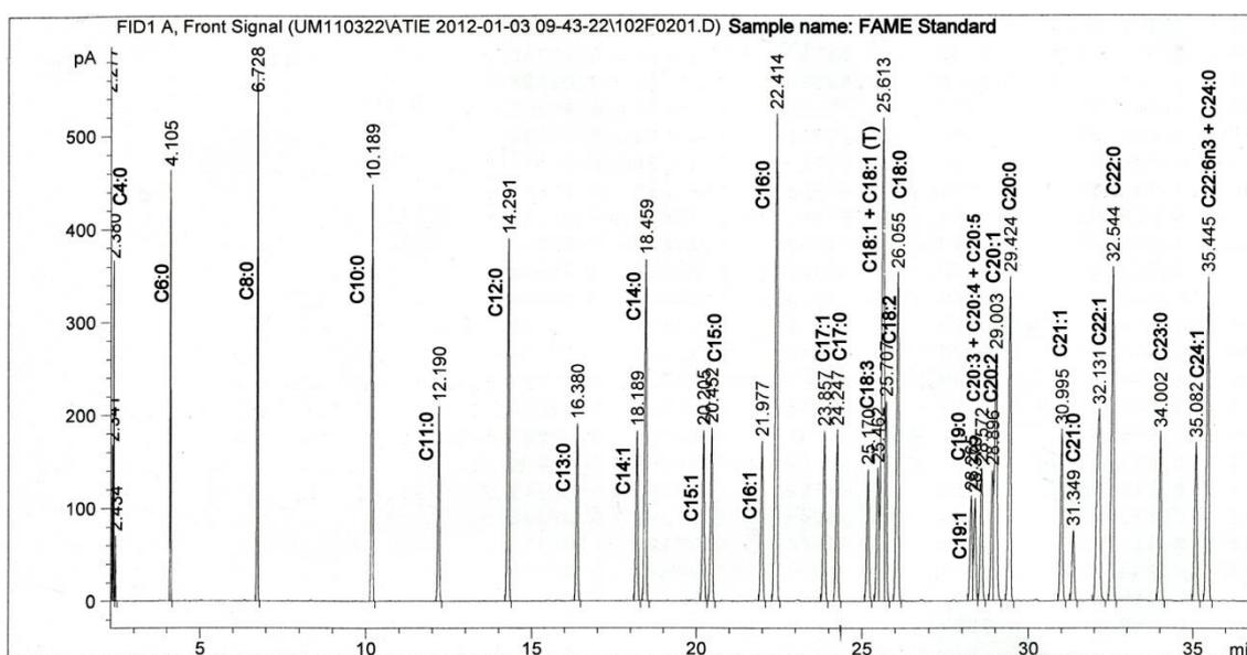
**Figure 3.23 :** GC chromatogram of FAME standard for ester content determination
