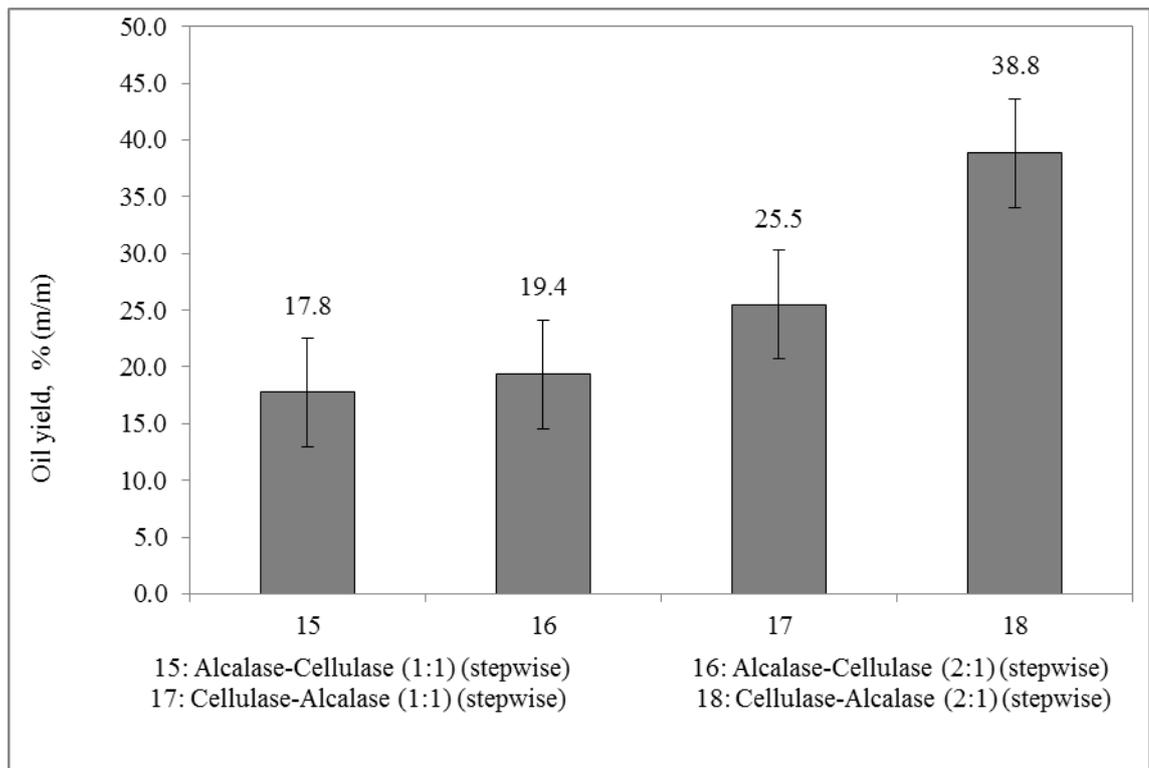
**Figure 3.2 :** Comparison of percentage (%) on oil yield by step-wise addition enzymatic extractions
