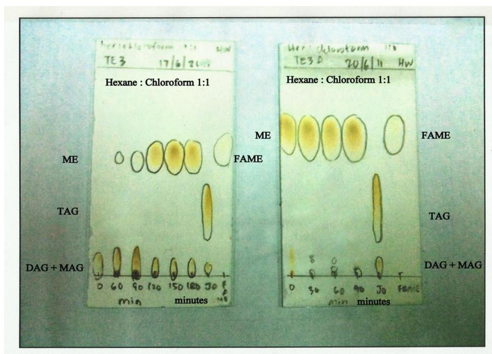
**Figure 3.11** : Thin-layer chromatography of double transesterification reaction
