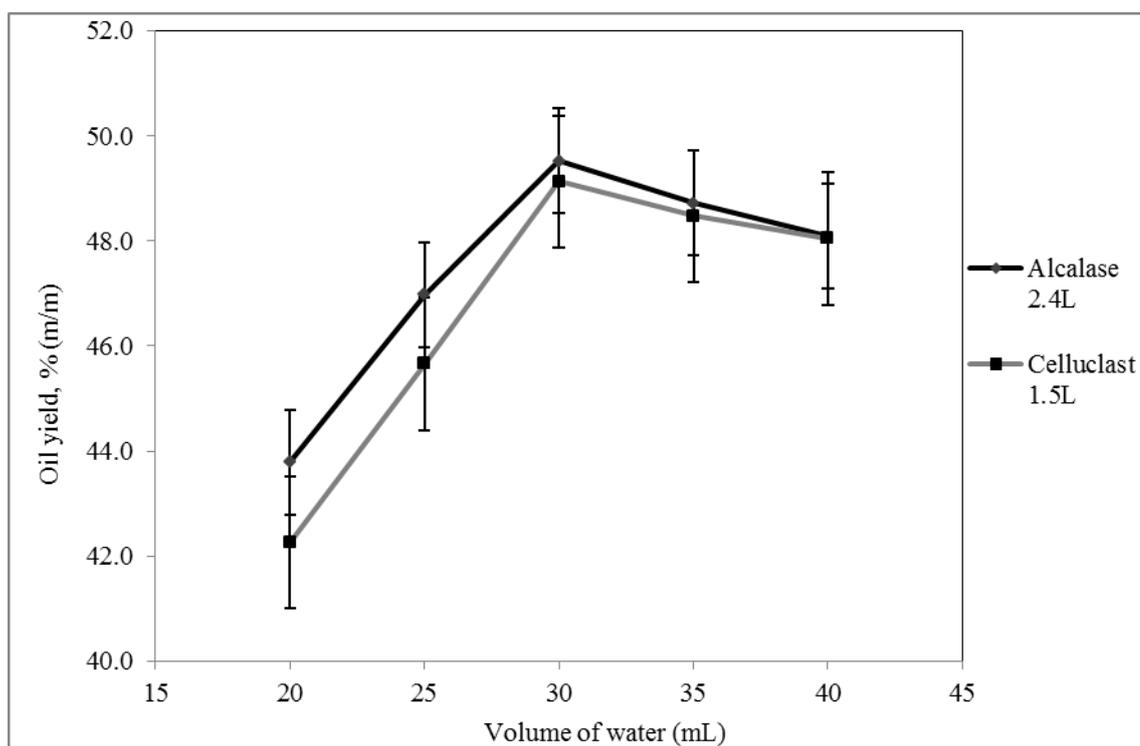
**Figure 3.9 :** Correlation between studies of water: seed ratio and percentage of oil yield, % obtained
