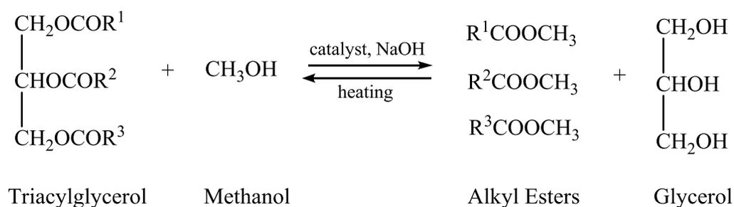
**Figure 3.10 :** Transesterification reaction between triacylglycerols in *Jatropha* oil by methanol in the presence of NaOH catalyst
