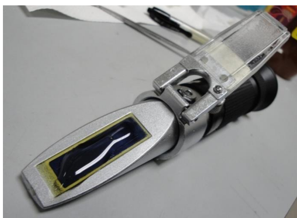
Figure 2.4: Prism of refractometer covered with honey.
