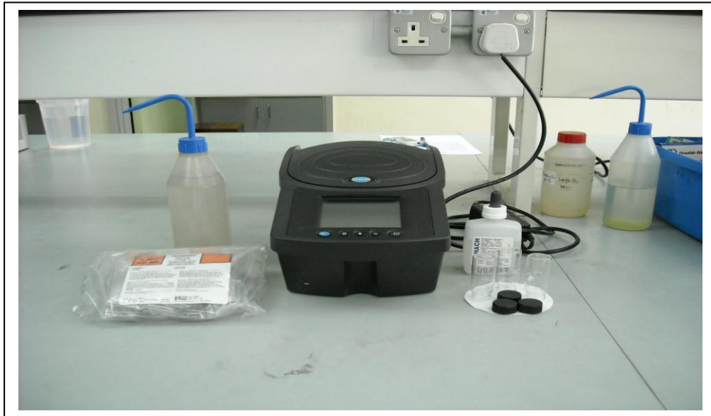
Plate 3.7: HACH Spectrometer for measuring water quality.
