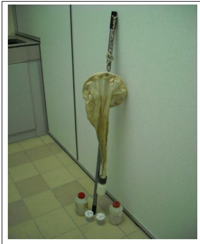
Plate 3.5: The apparatus for sampling (plankton net, bottles and vials)
