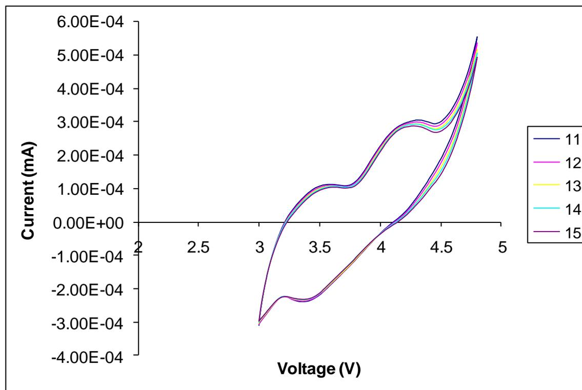
Cyclic voltammetry of 1.0 wt.% of ZnO coated sample (11th-15th cycles)
