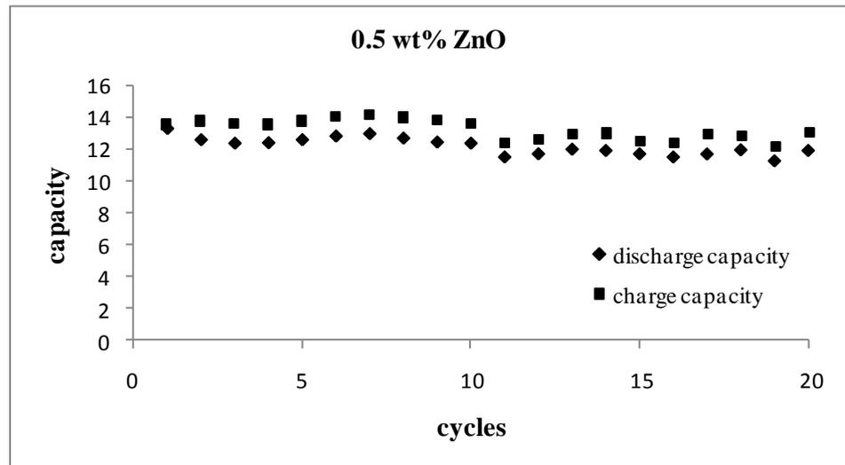
Fig. 6.18: Charge-discharge studies of 0.5 wt% ZnO coated LiNiVO<sub>4</sub>
