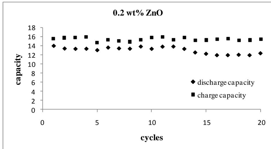
**Fig. 6.17:** Charge-discharge studies of 0.2 wt% ZnO coated LiNiVO<sub>4</sub>
