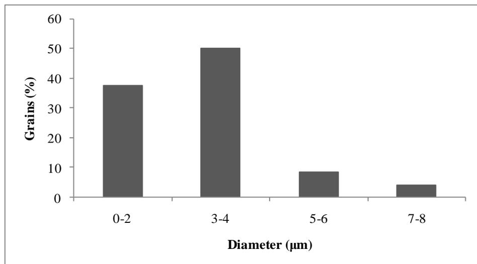
**Fig. 6.13: Distribution of diameter of 1.0 wt.% ZnO coated LiNiVO<sub>4</sub>**
