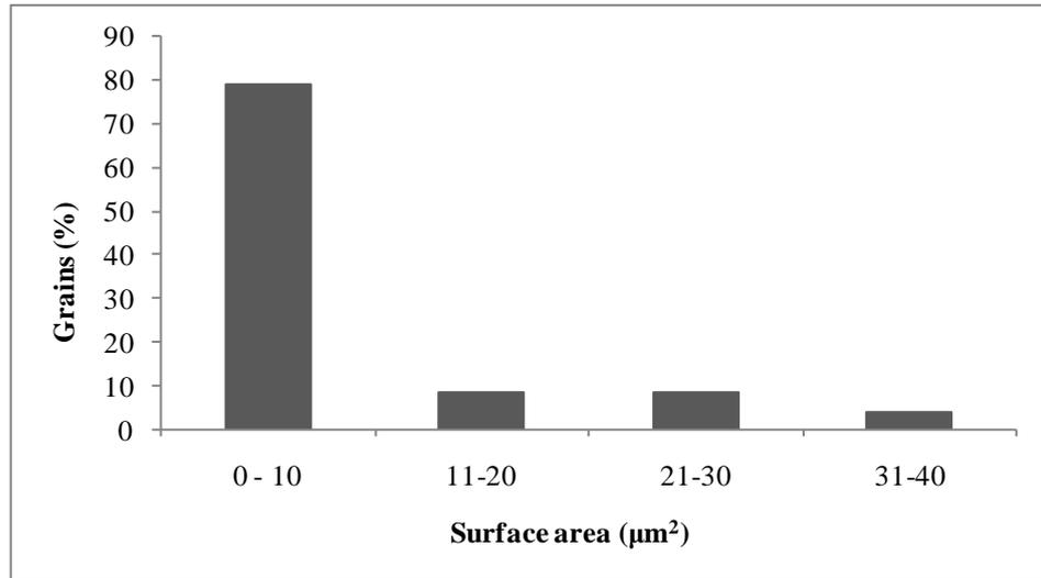
**Fig. 6.12: Distribution of surface area of 1.0 wt.% ZnO coated LiNiVO<sub>4</sub>**
