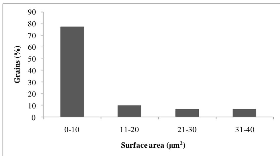
**Fig. 6.9: Distribution of surface area of 0.5 wt.% ZnO coated LiNiVO<sub>4</sub>**
