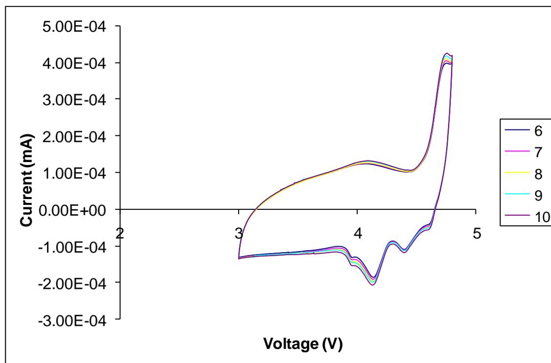
Cyclic voltammetry of 0.2 wt.% of ZnO coated sample (6th-10th cycles)
