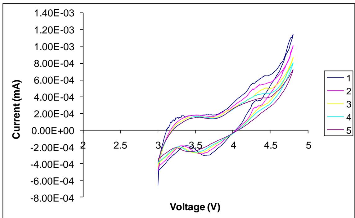
Cyclic voltammetry of 1.0 wt.% of ZnO coated sample (1st-5th cycles)
