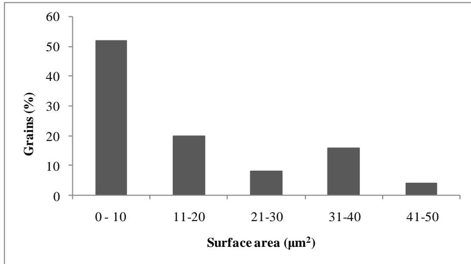
**Fig. 6.6: Distribution of surface area of 0.2 wt.% ZnO coated LiNiVO<sub>4</sub>**
