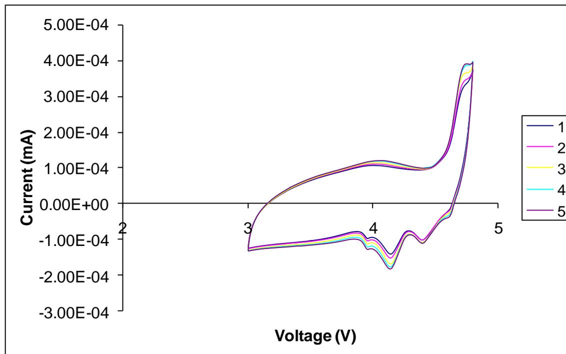
Cyclic voltammetry of 0.2 wt.% of ZnO coated sample (1st-5th cycles)
