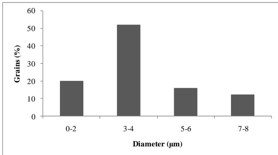
**Fig. 6.7: Distribution of diameter of 0.2 wt.% ZnO coated LiNiVO<sub>4</sub>**
