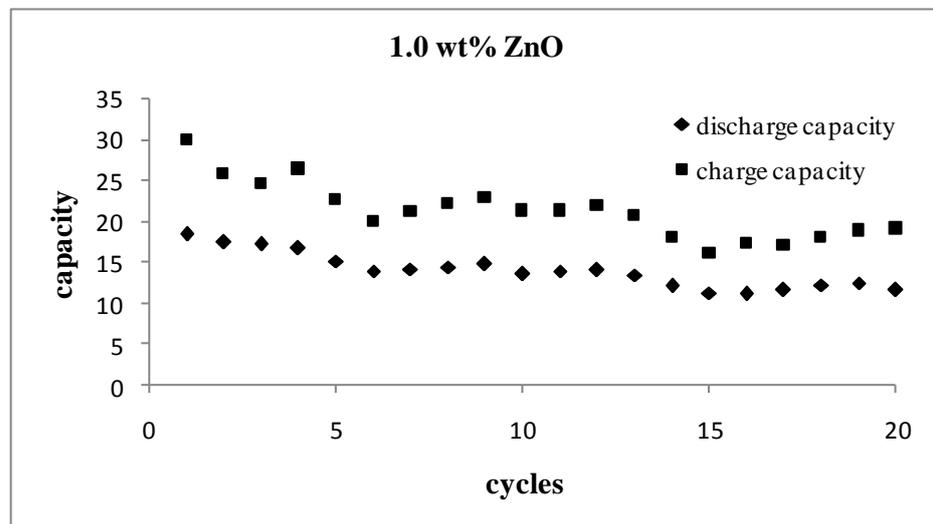
Fig. 6.19: Charge-discharge studies of 1.0 wt% ZnO coated LiNiVO<sub>4</sub>
