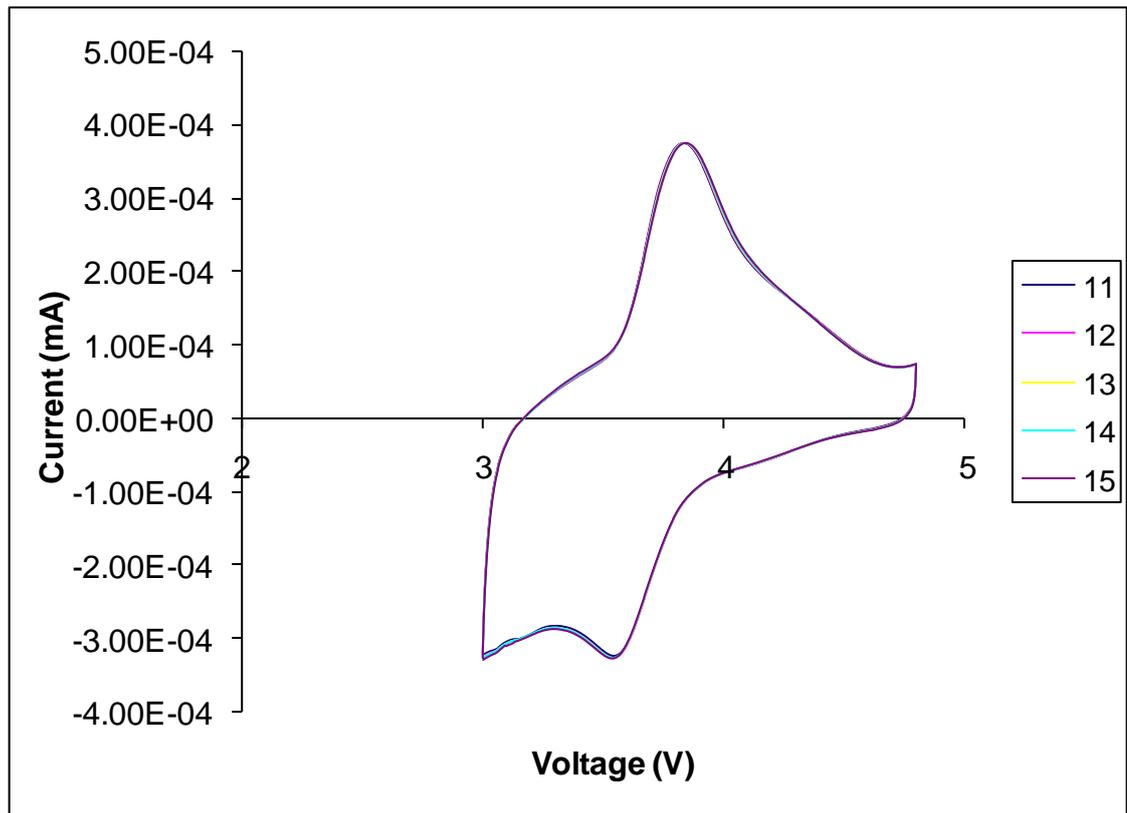
Cyclic voltammetry of 0.5 wt.% of ZnO coated sample (11th-15th cycles)
