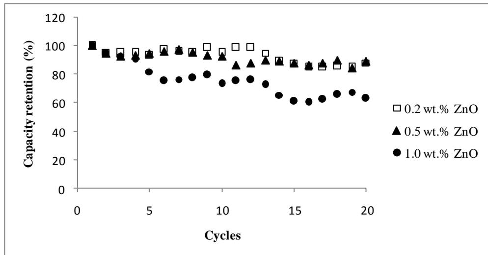
Fig. 6.21: Capacity retention of ZnO coated LiNiVO<sub>4</sub>
