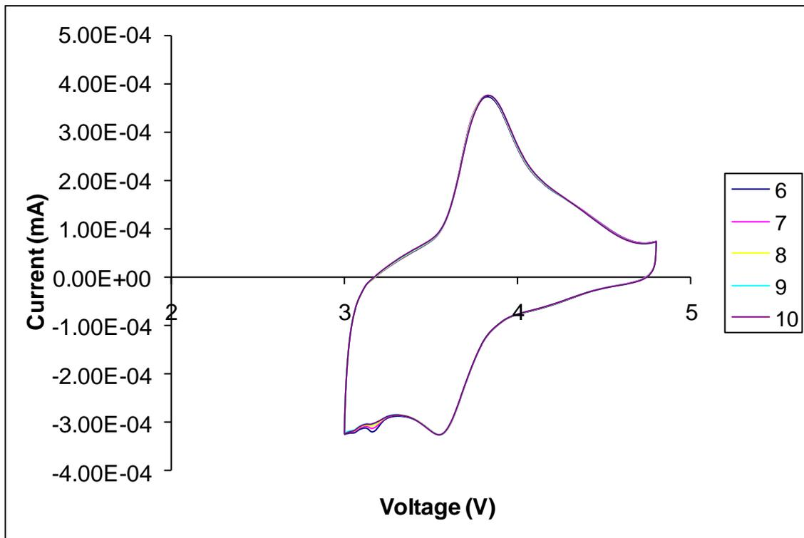
Cyclic voltammety of 0.5 wt.% of ZnO coated sample (6th-10th cycles)
