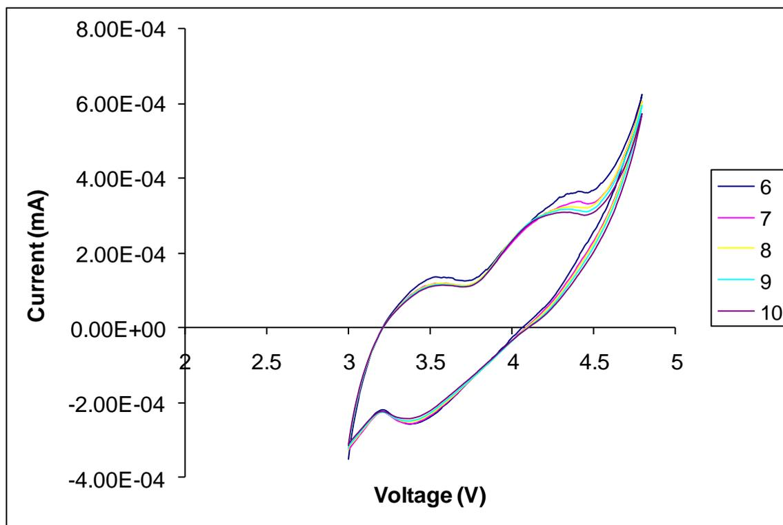
Cyclic voltammetry of 1.0 wt.% of ZnO coated sample (6th-10th cycles)
