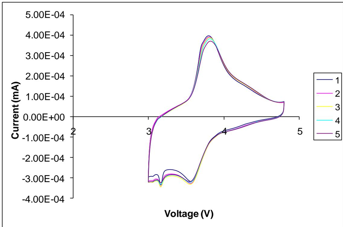
Cyclic voltammety of 0.5 wt.% of ZnO coated sample (1st-5th cycles)
