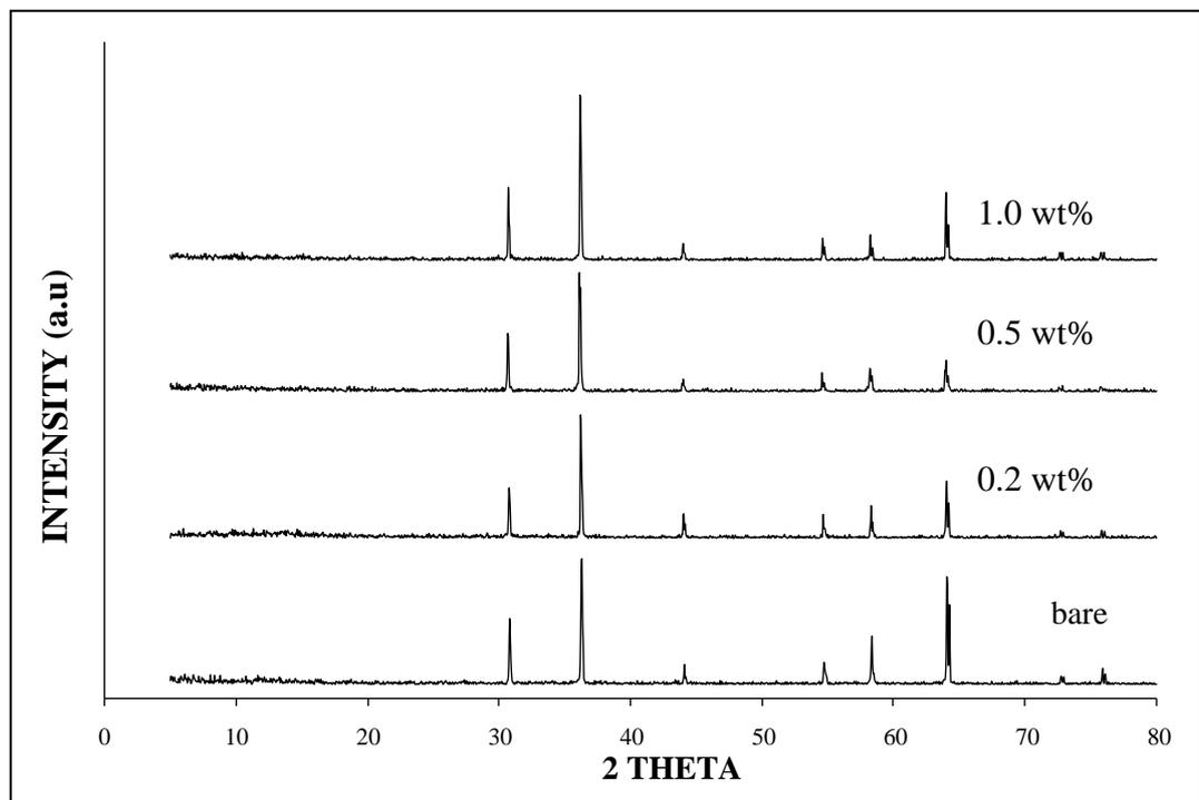
**Fig.6.1: XRD of ZnO coated LiNiVO<sub>4</sub> at sintering temperature of 700 °C**
