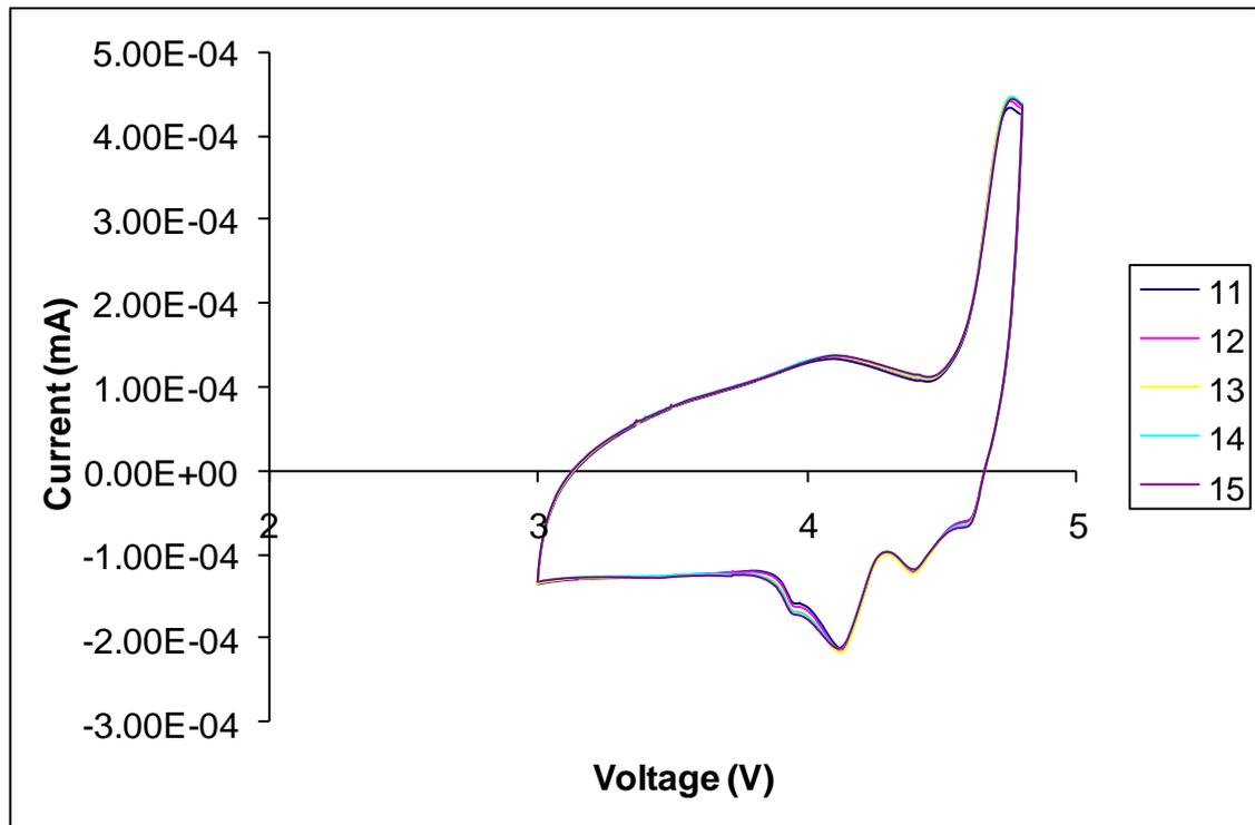
Cyclic voltammetry of 0.2 wt.% of ZnO coated sample (11th-15th cycles)
