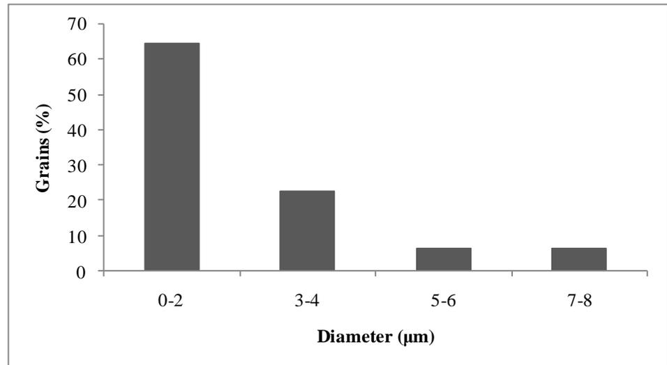
**Fig. 6.10: Distribution of diameter of 0.5 wt.% ZnO coated LiNiVO<sub>4</sub>**
