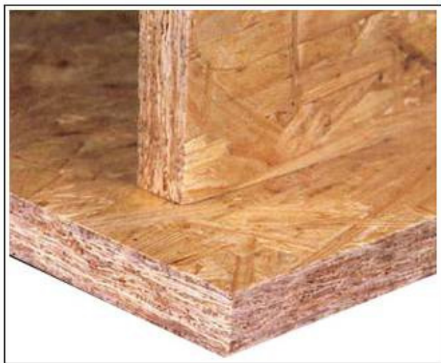
Figure 1.5: Oriented strand board that made from a mixture of dried small wood chips, glue and additives
