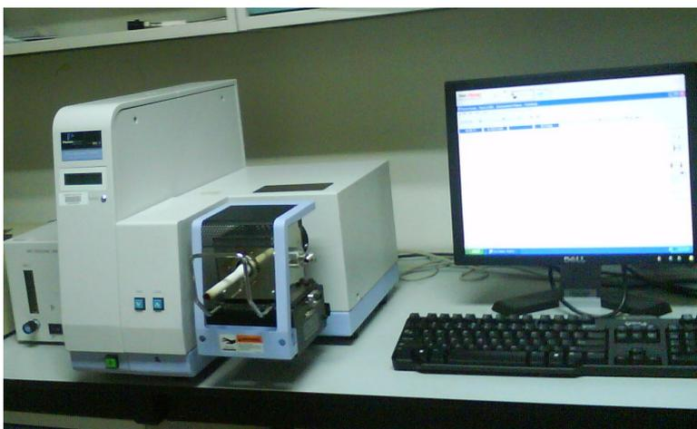
Figure 2.3: Perkin-Elmer TGA7
