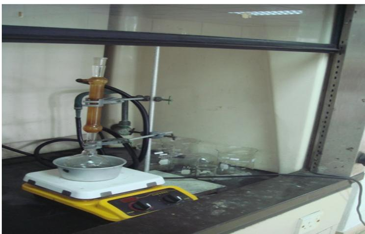
Figure 2.1: Apparatus set-up for the synthesis of chromium(III) complexes
