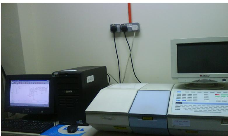
Figure 2.2: Perkin Elmer Fourier Transform Infrared (FT-IR)
