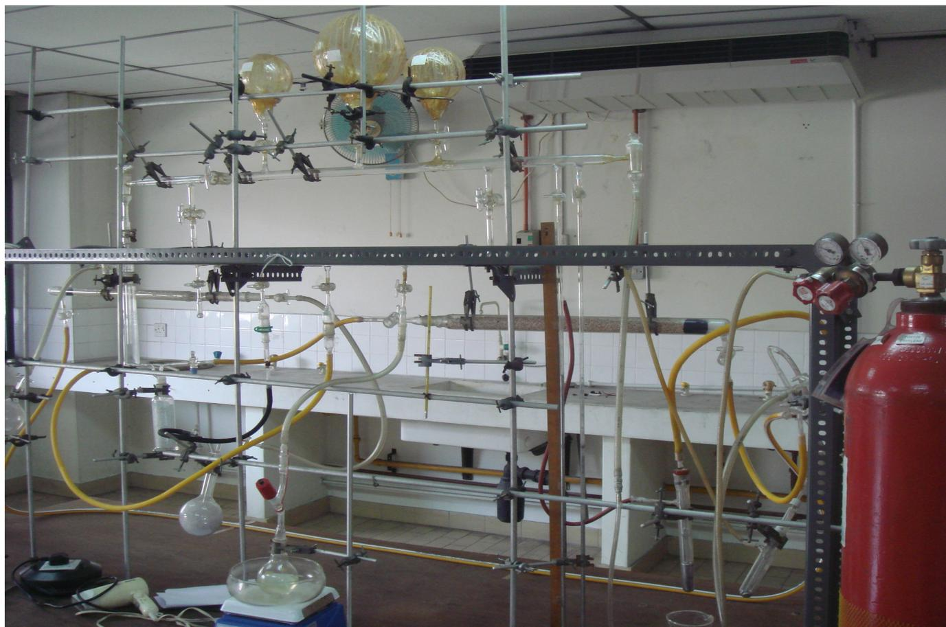
Figure 2.4: Polymerization gas line with constant volume set-up
