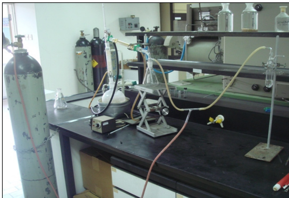
Figure A1: Apparatus set-up for toluene distillation
