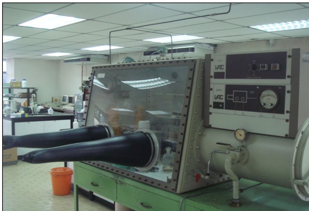
Figure A3: Dry box for the preparation of catalyst and cocatalyst mixture
