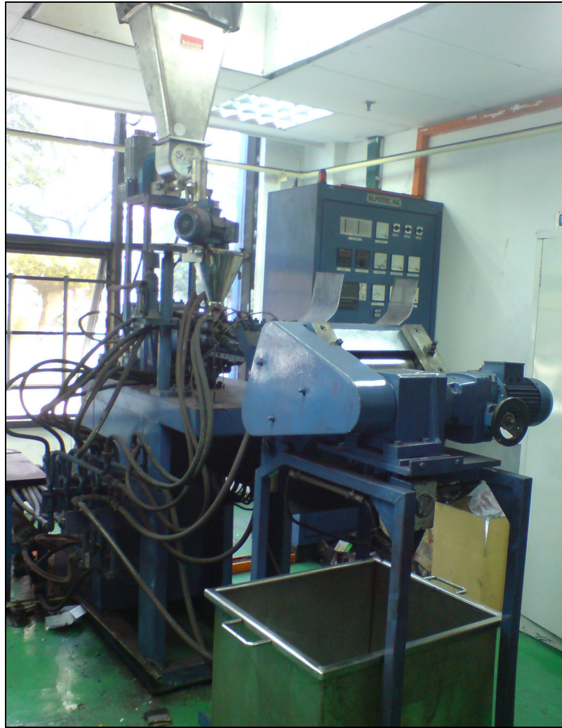
Figure 2.11 Extruder was used to melt the mixture and extrude the mixture of resin, magnetite pigment, wax and charge control agent.
