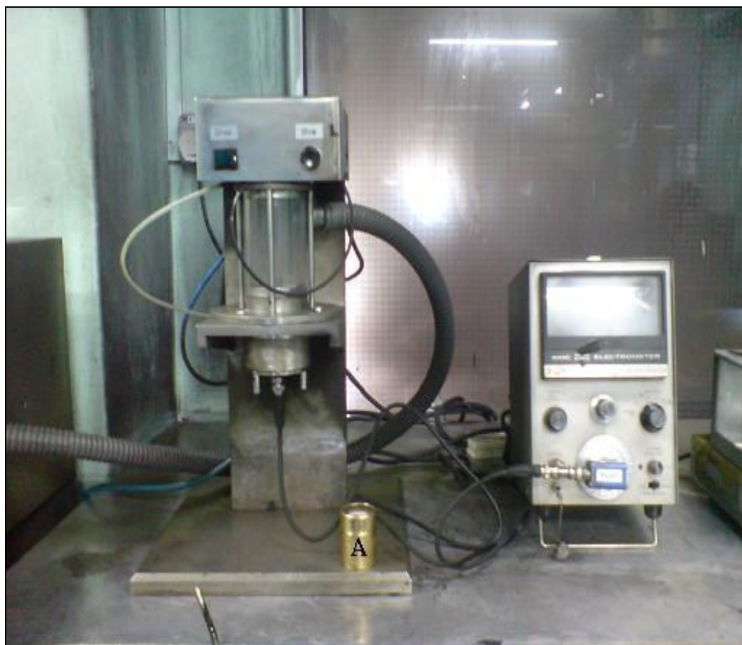
Figure 2.17 Keithley Instruments 610C solid state electrometer (A: sample container)
