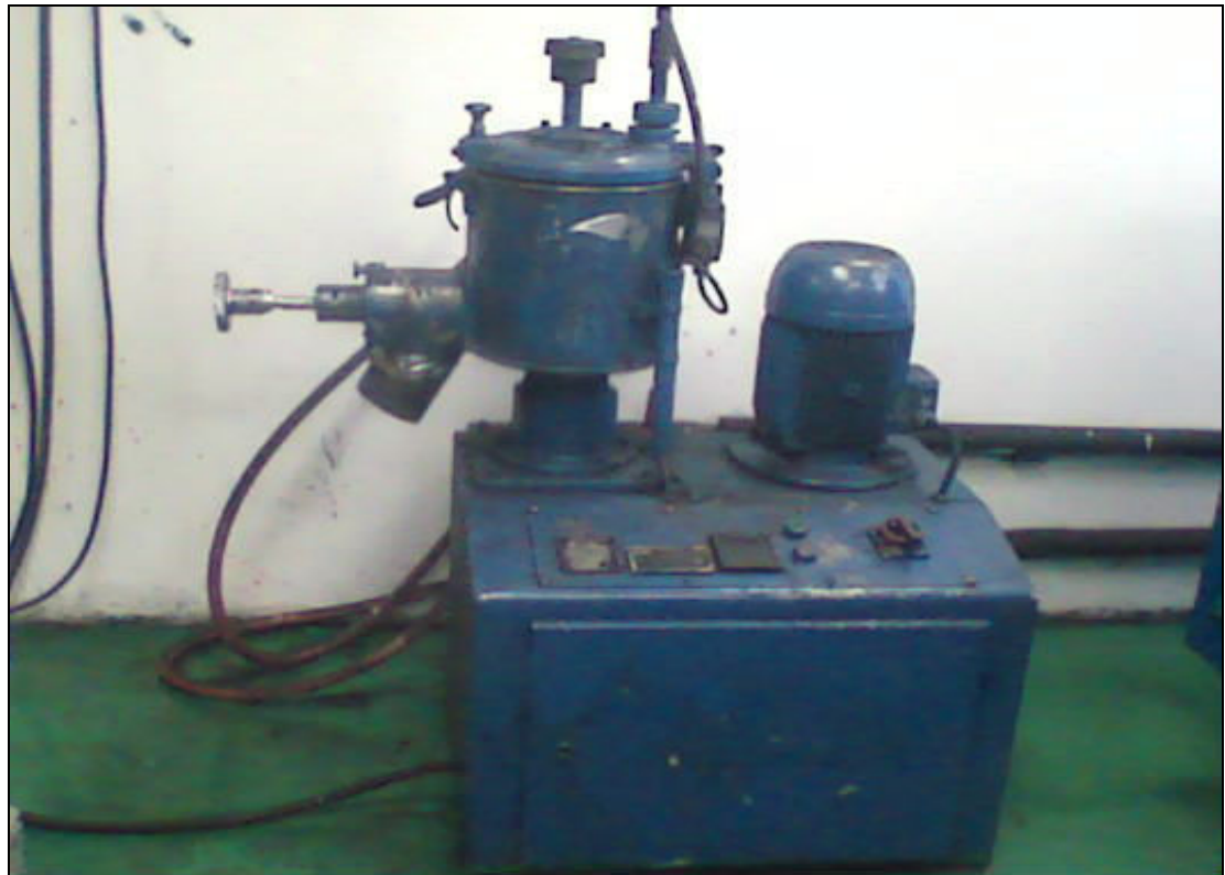
Figure 2.10 Mixer used to mix the resin, magnetite pigment, wax and charge control agent.
