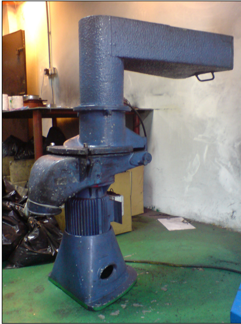
Figure 2.12 Crusher was used to crush down the extruded mixture into rough powder
