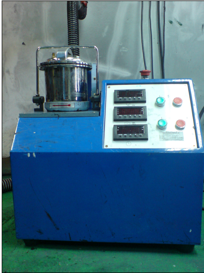
Figure 2.14 Blender was used to blend the toner powder together with magnetite pigment, silica and zinc stearate to produce a finished toner.
