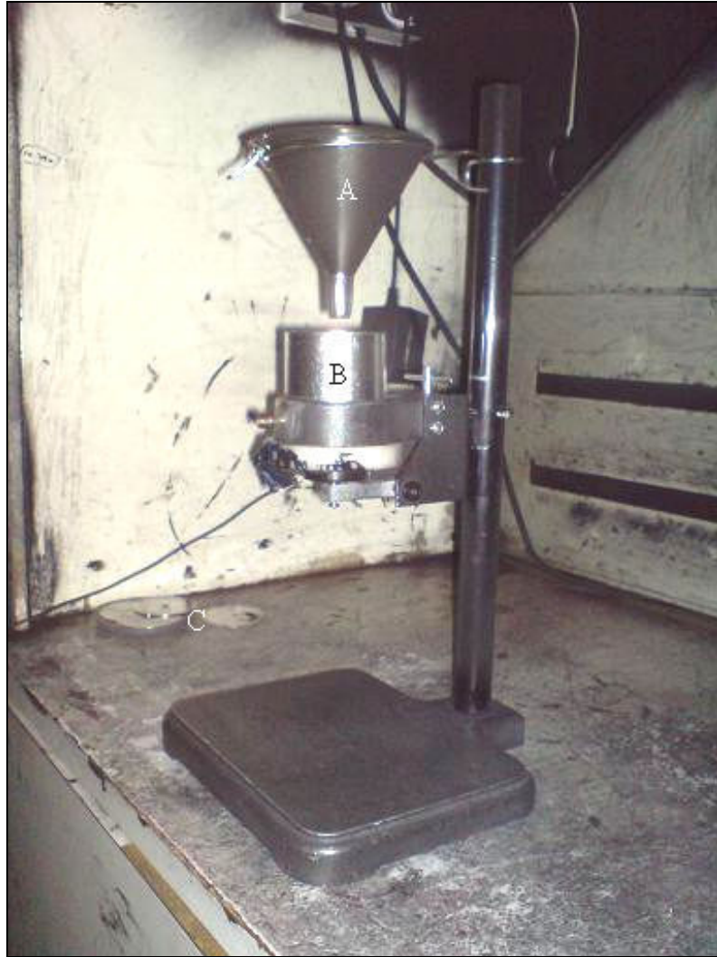
Figure 2.16 Flowability equipment (A: sample hopper, B: sample container, C: disc with different pore size)
