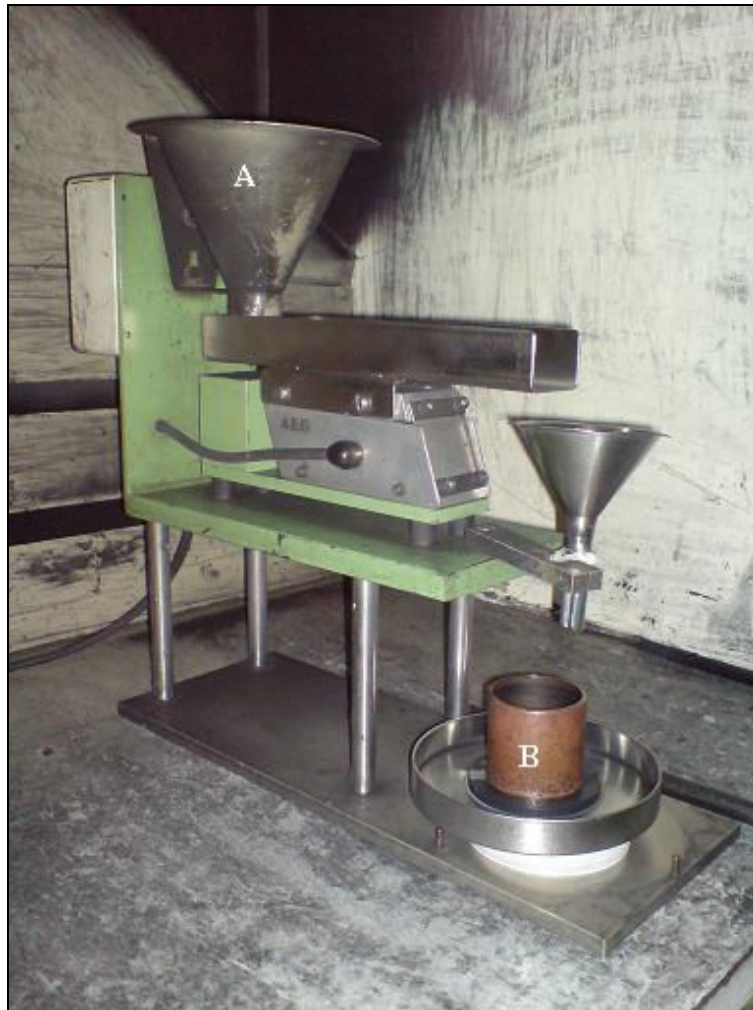
Figure 2.15 Apparent density equipment (A: sample hopper, B: sample container)
