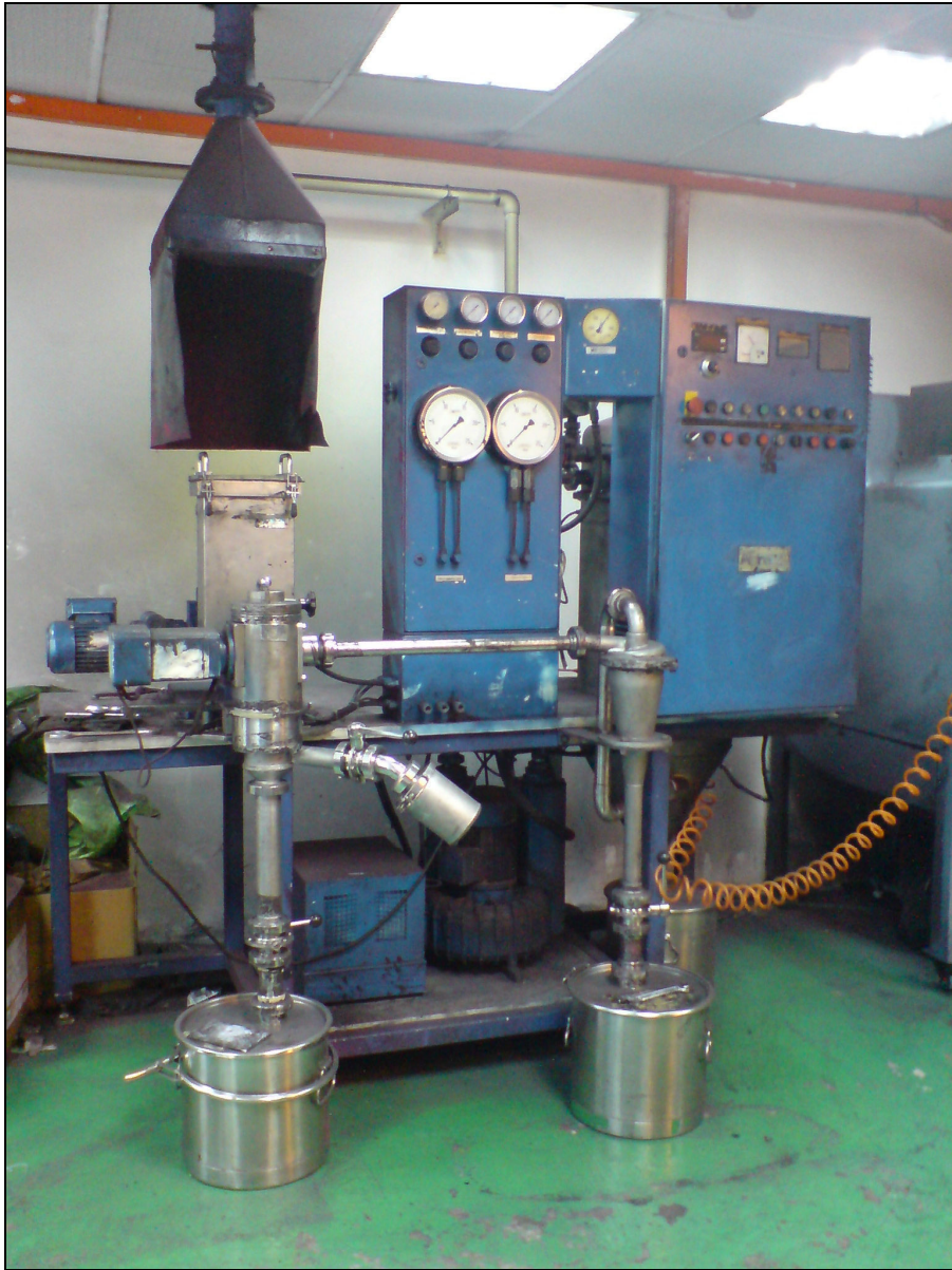
Figure 2.13 Miller was used to reduce the size of the rough powder, wherein classifier was used to produce toner powder in more even sizes.
