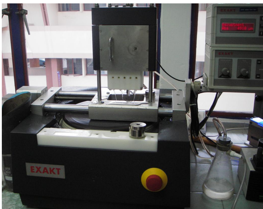
Figure 3.9 Grinding Machine (EXAKT 400 CS) - set up with sand paper.
