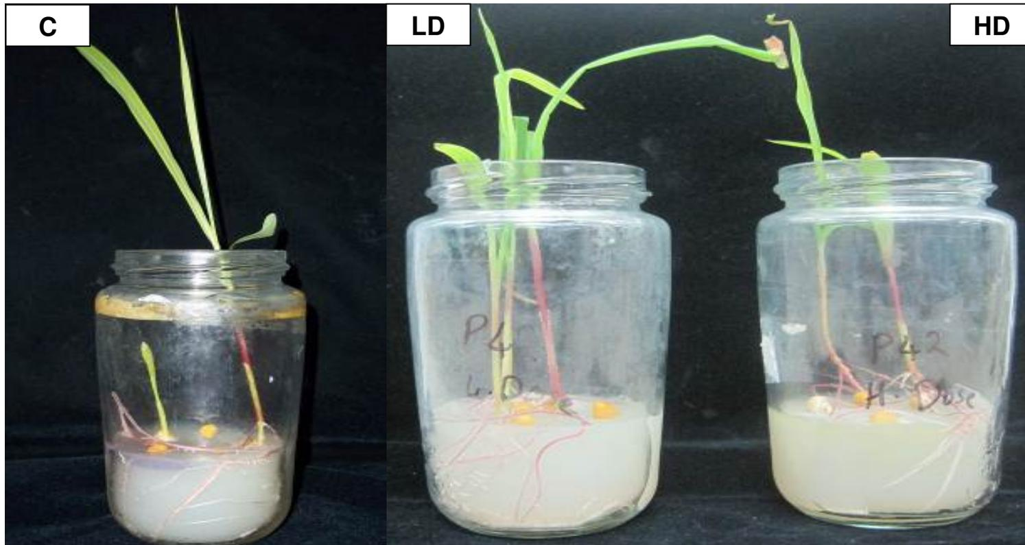
**Plate 4.34:** Phytotoxicity test. Germination and growth of Maize seeds after 10 days of incubation on ISP2 agar 2% (w/v) at  $28 \pm 2^\circ\text{C}$
