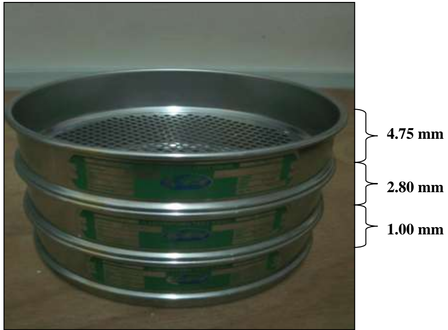
Plate 3.3: A set of nested sieve.
