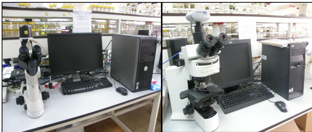
Plate 3.6: a) Light Microscopy Nikon Eclipse TS100 b) Light Microscopy Olympus BX5.
