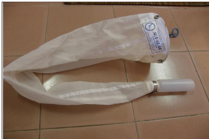
Plate 3.5: 30µm wire mesh plankton net.
