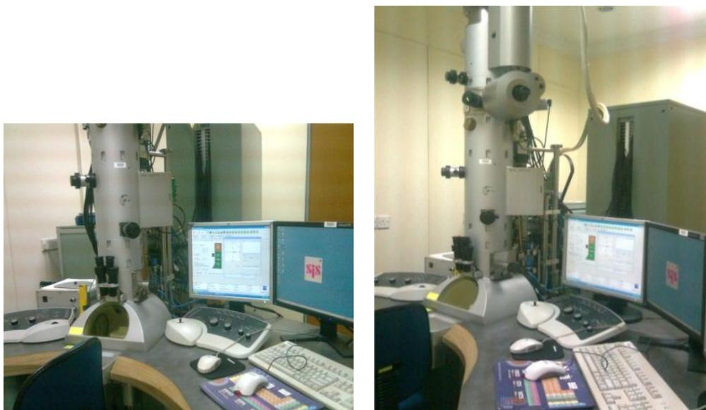
Figure 3.14 The Transmission Electron Microscopy (TEM) analyser, LEO-Libra 120
