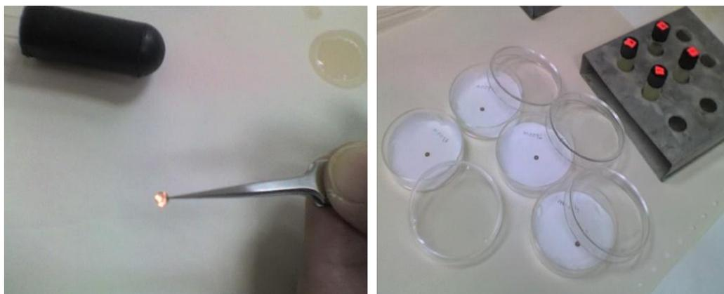
**Figure 3.16** The etching preparation for TEM analysis
