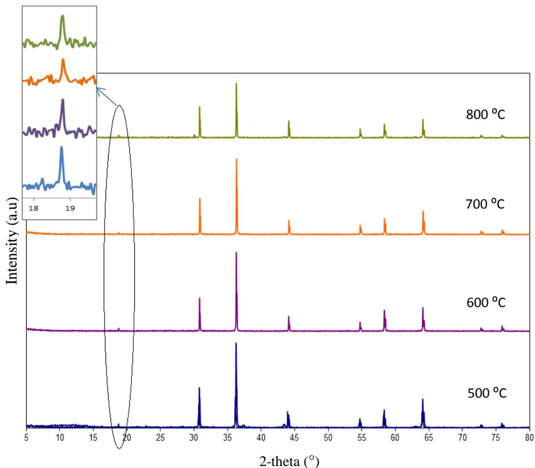
**Figure 4.2: XRD pattern for the ( $\text{LiNiVO}_4$ - SG) system**
