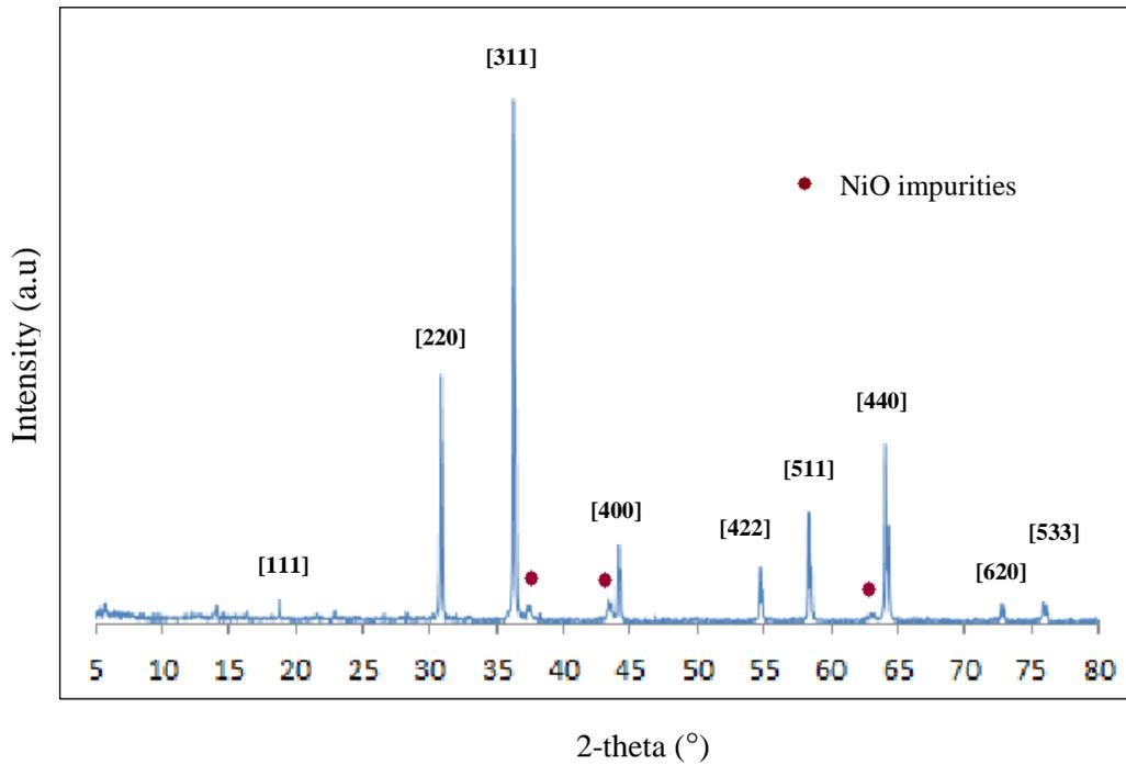
**Figure 4.1:** Mixed phase for the ( $\text{LiNiVO}_4$ - SG) system at 500 °C
