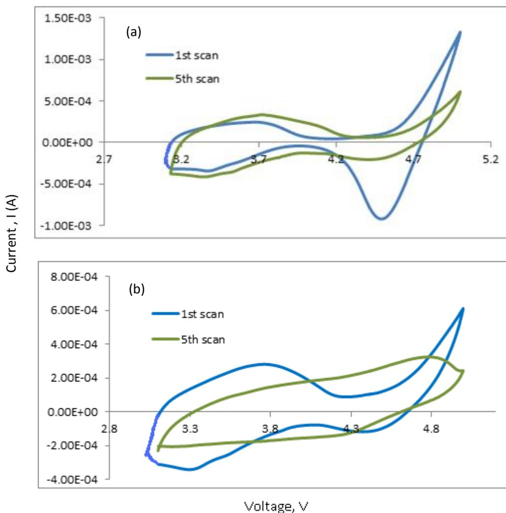
**Figure 4.7:** Cyclic voltammograms for Li/  $\text{LiNiVO}_4$ - SG electrode system in  $1 \text{ mol dm}^{-1} \text{LiPF}_6$  in 1:2 by (vol/ vol%) EC/DMC at scan rate of  $1 \text{ mV/s}$  (a) cathode sintered at  $600 \text{ }^\circ\text{C}$ ; (b) cathode sintered at  $800 \text{ }^\circ\text{C}$
