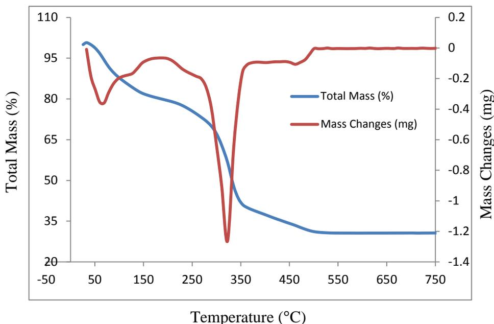
**Figure 4.3 TGA and DTGA curve of the  $\text{LiNiVO}_4$ – SG precursor**
