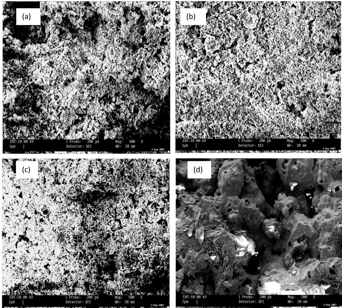
**Figure 4.4:** Surface morphology of  $\text{LiNiVO}_4$ -SG system (a)  $\text{LiNiVO}_4$ -SG at 500 °C; (b)  $\text{LiNiVO}_4$ -SG at 600 °C; (c)  $\text{LiNiVO}_4$ -SG at 700 °C; (d)  $\text{LiNiVO}_4$ -SG at 800 °C with 500X magnification
