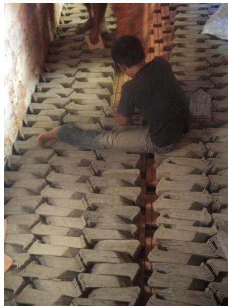
Figure 4.13: The arrangement of green Singgora tiles inside the kiln's chamber Source: Field study (2013)
