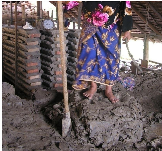
Figure 4.3: The clay is kneaded with foot Source: Field study (2013)
