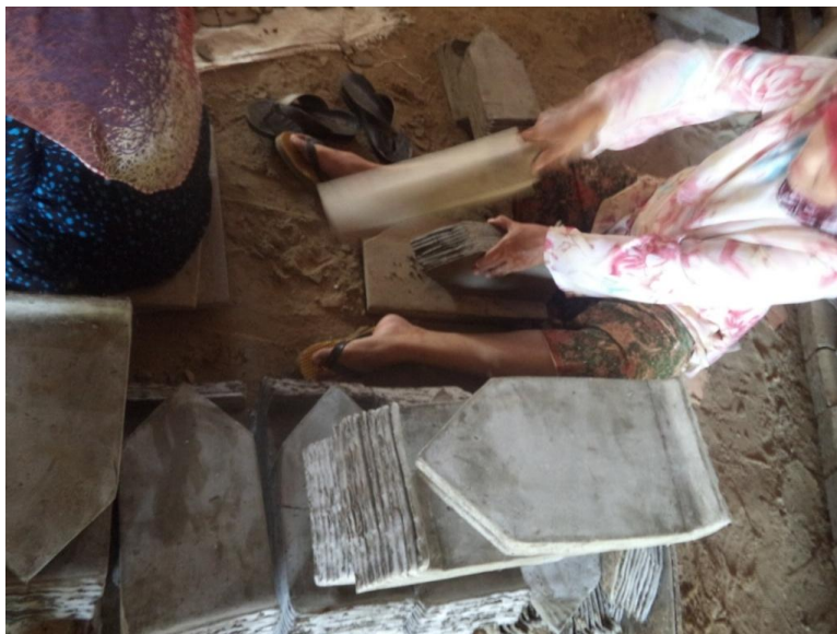
Figure 4.10: Each side of dry green tiles are banging with paddle Source: Field study (2013)
