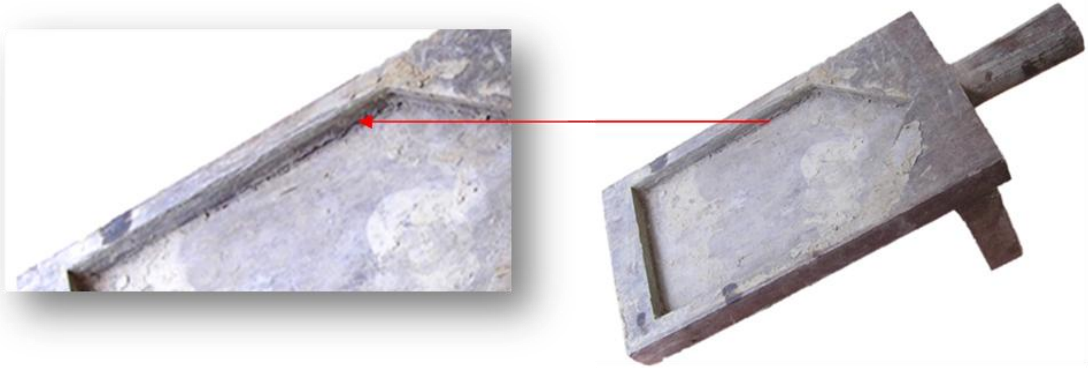
Figure 4.27: The dried clay and less joint between the corner and base of mould Source: Field study (2013)
