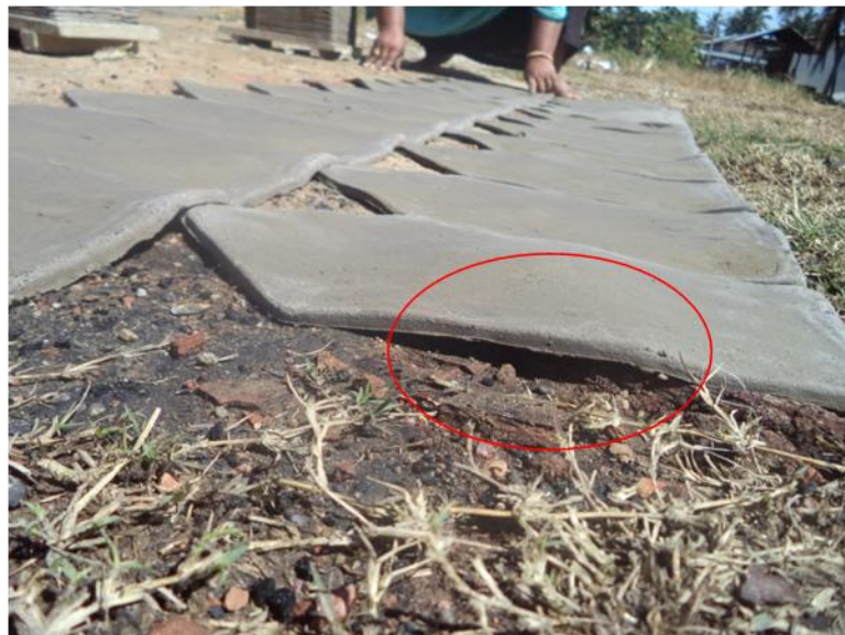
Figure 4.30: Uneven shaped of green tiles due to the improper drying area Source: Field study (2013)
