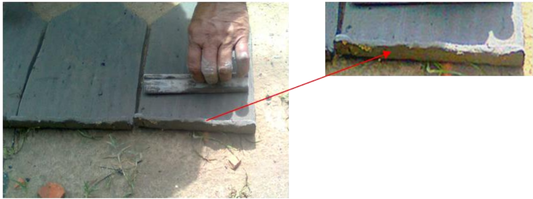
Figure 4.26: The mark of finger along the edge of hook Source: Field study (2013)
