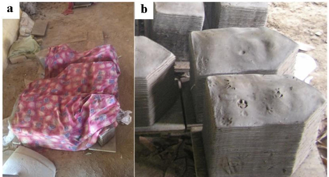
Figure 4.6: The green tiles are covered with cloth (a) and footprint by livestock (b) Source: Field study (2013)
