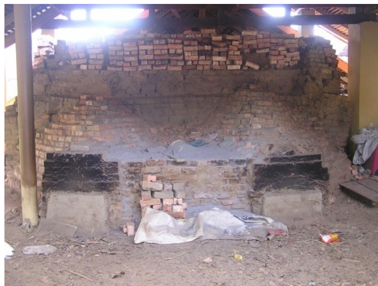
Figure 4.15: The two fire holes were blocked up to allow the kiln cool naturally Source: Field study (2013)
