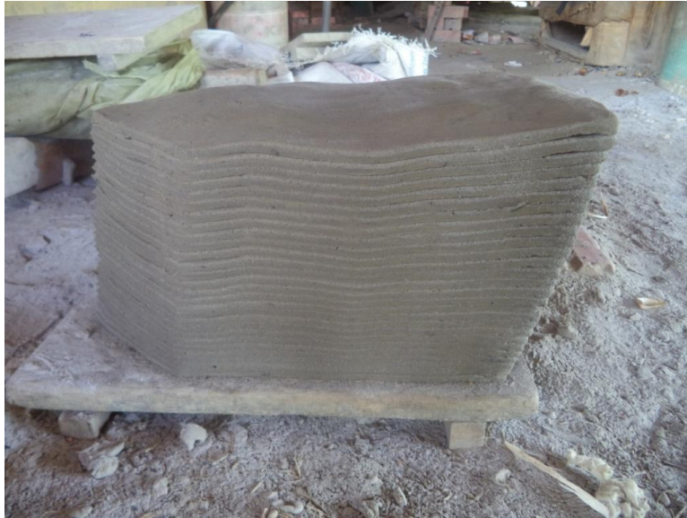
Figure 4.5: The back area of green tiles is thicker than front Source: Field study (2013)
