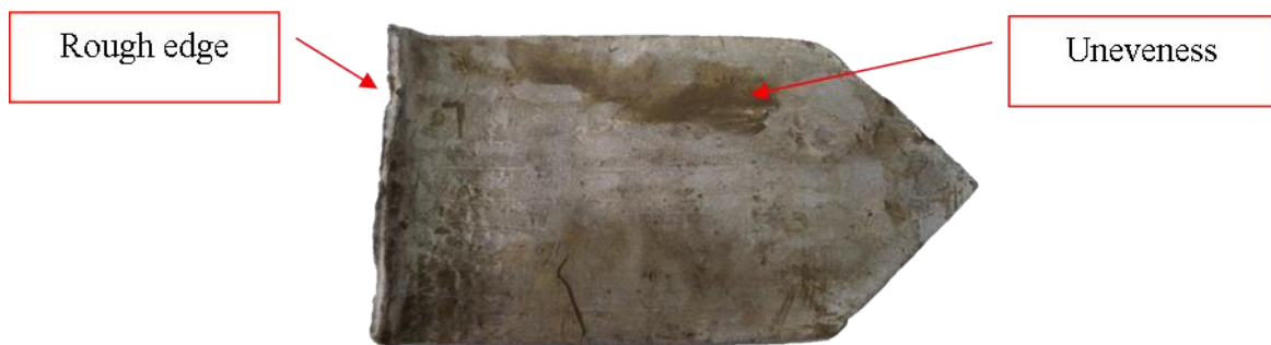
Figure 4.25: Rough edge and unevenness surface of green tile Source: Field study (2013)
