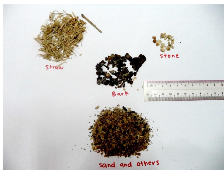
Figure 4.37: Types of impurities in five pieces of green tiles Source: Field study (2013)
