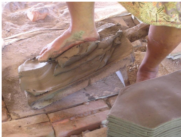
Figure 4.4: The clay is kneaded with foot above the surface of wooden mould Source: Field study (2013)
