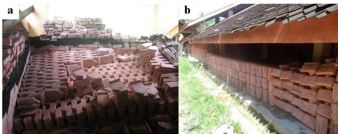
Figure 4.16: Singgora tiles in the kiln (a) and in the edge of factory (b) Source: Field study (2013)
