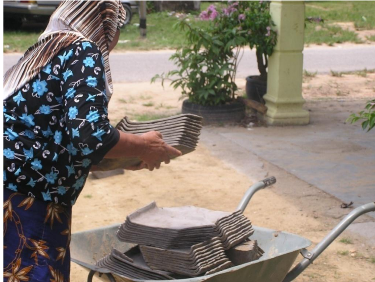
Figure 4.9: The dry green tiles are stacks onto a barrow Source: Field study (2013)
