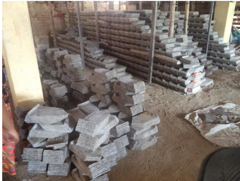
Figure 4.11: The dried green tiles were stacked without rack in the factory Source: Field study (2013)
