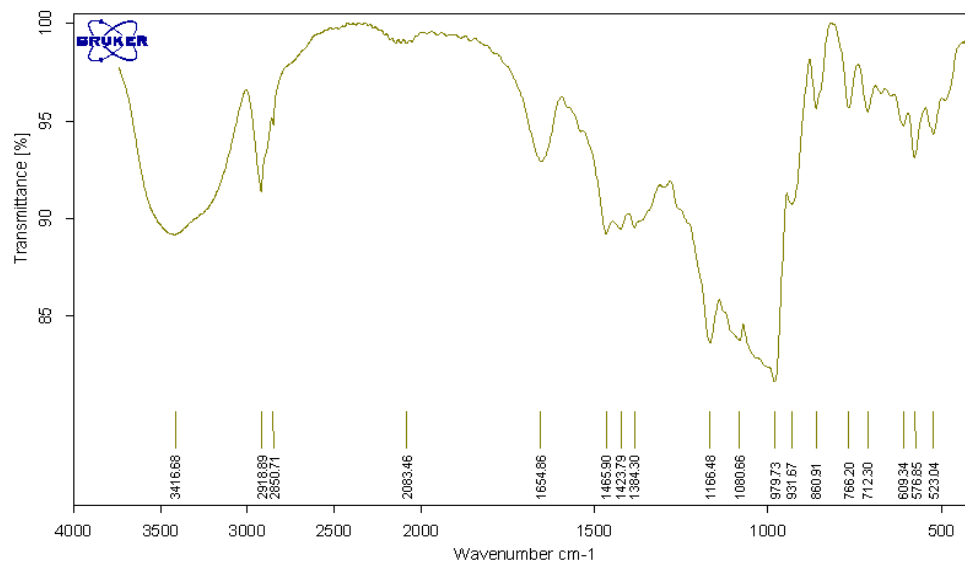
Figure 4.3: FT-IR spectra of pregelatinised sago starch PS2.
