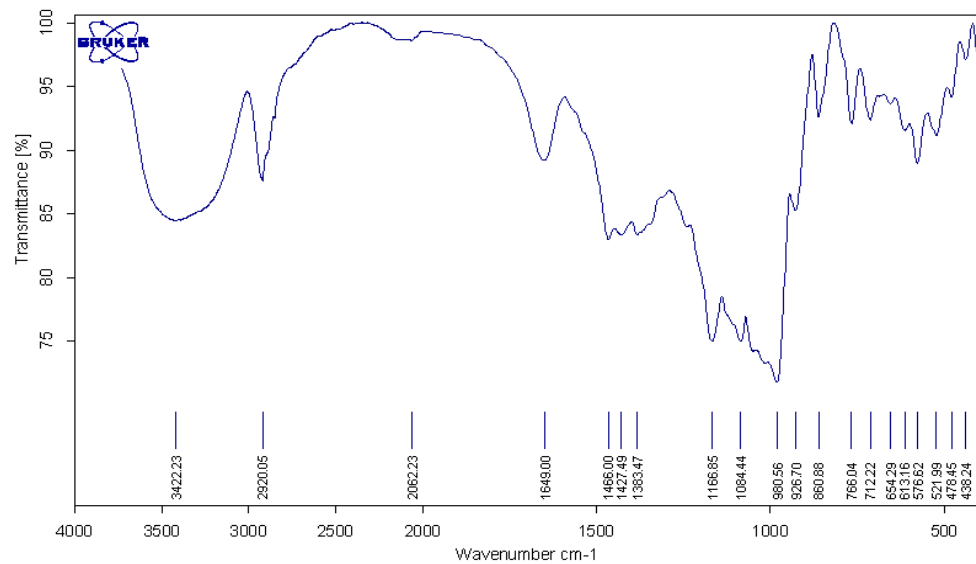
Figure 4.2: FT-IR spectra of pregelatinised sago starch PS1.
