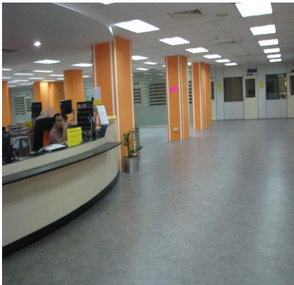
Figure 5.28: Lack of tactile path inside library
