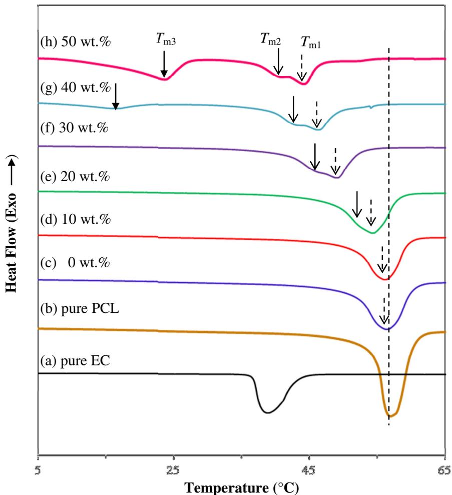
**Fig. 4.6** Magnified DSC thermograms of PCL-NH<sub>4</sub>SCN-EC films added with 0 to 50 wt.% EC, showing  $T_m$ .
