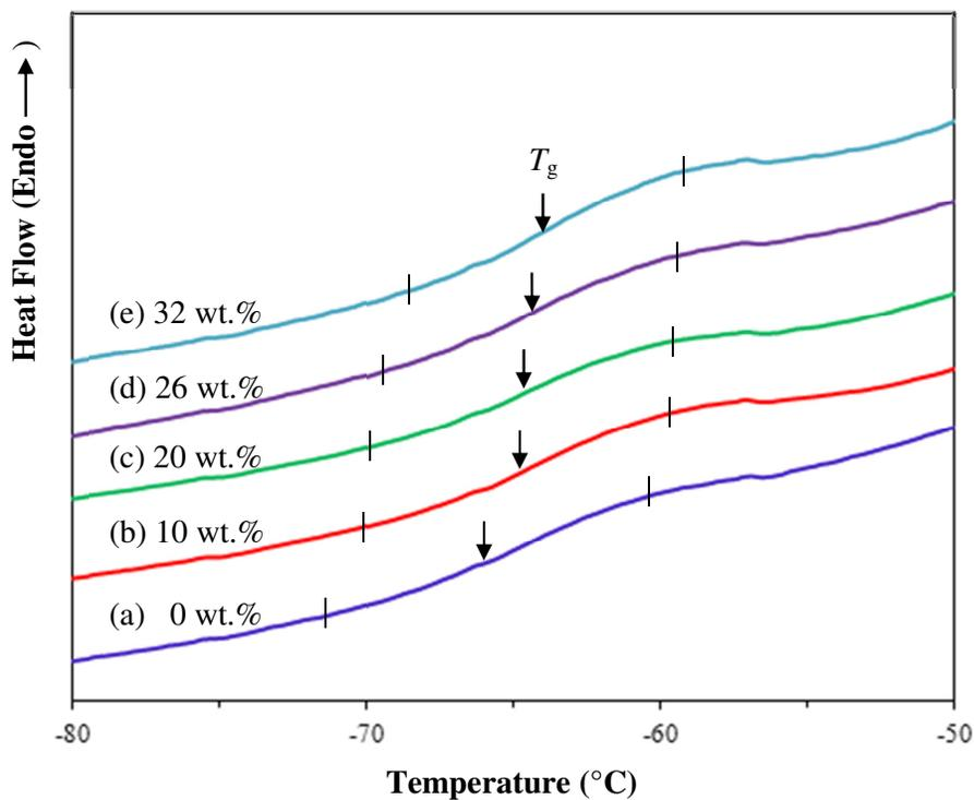
**Fig. 4.2** Magnified DSC thermograms of PCL-NH<sub>4</sub>SCN films added with 0 to 32 wt.% NH<sub>4</sub>SCN, showing  $T_g$ .
