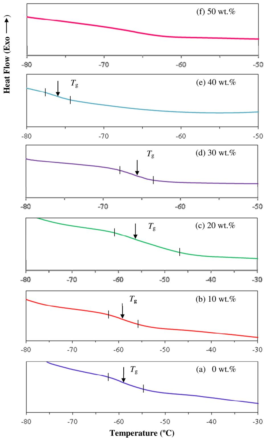
**Fig. 4.5** Magnified DSC thermograms of PCL-NH<sub>4</sub>SCN-EC films added with 0 to 50 wt.% EC, showing  $T_g$ .
