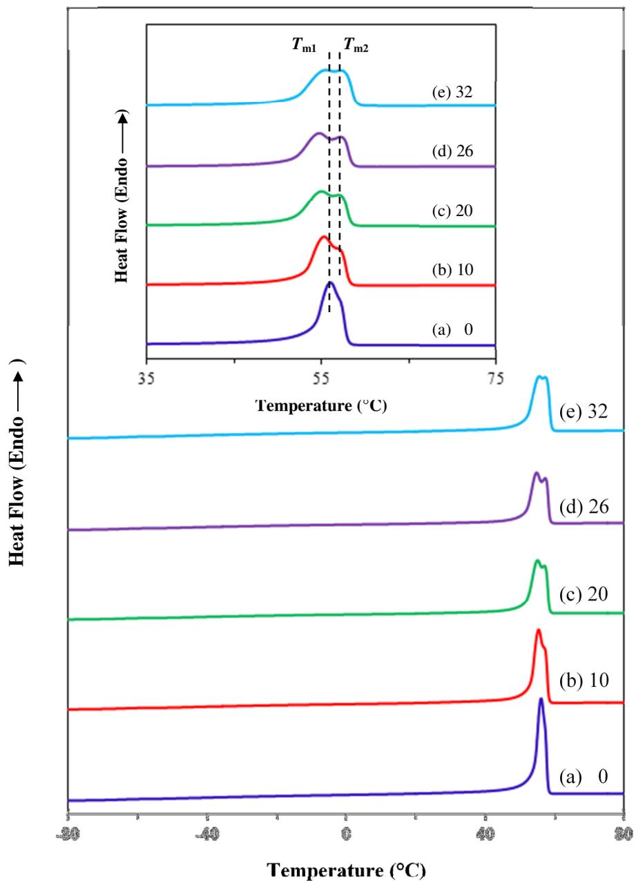
**Fig. 4.1** DSC thermograms of PCL-NH<sub>4</sub>SCN films added with 0 to 32 wt.% NH<sub>4</sub>SCN. Inset shows the magnified thermograms indicating  $T_m$ .
