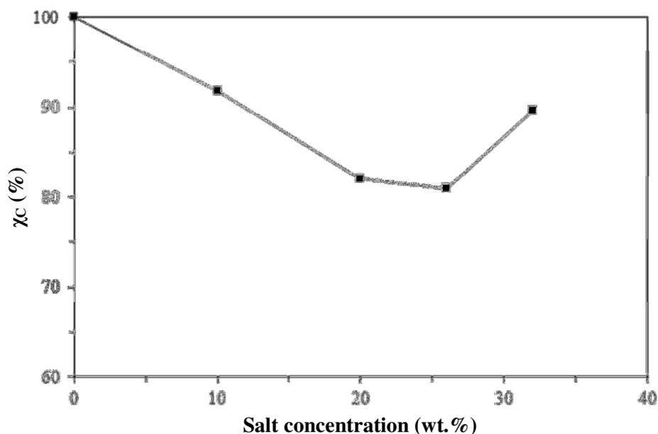
**Fig. 4.3** Relative degree of crystallinity as a function of salt content for PCL-NH<sub>4</sub>SCN films added with 0 to 32 wt.% NH<sub>4</sub>SCN.
