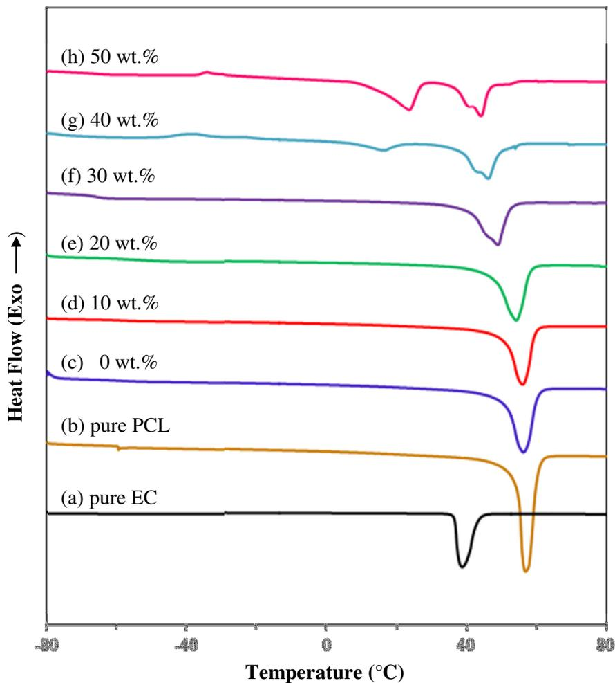
**Fig. 4.4** DSC thermograms of pure EC, pure PCL and PCL-NH<sub>4</sub>SCN-EC films added with 0 to 50 wt.% EC.
