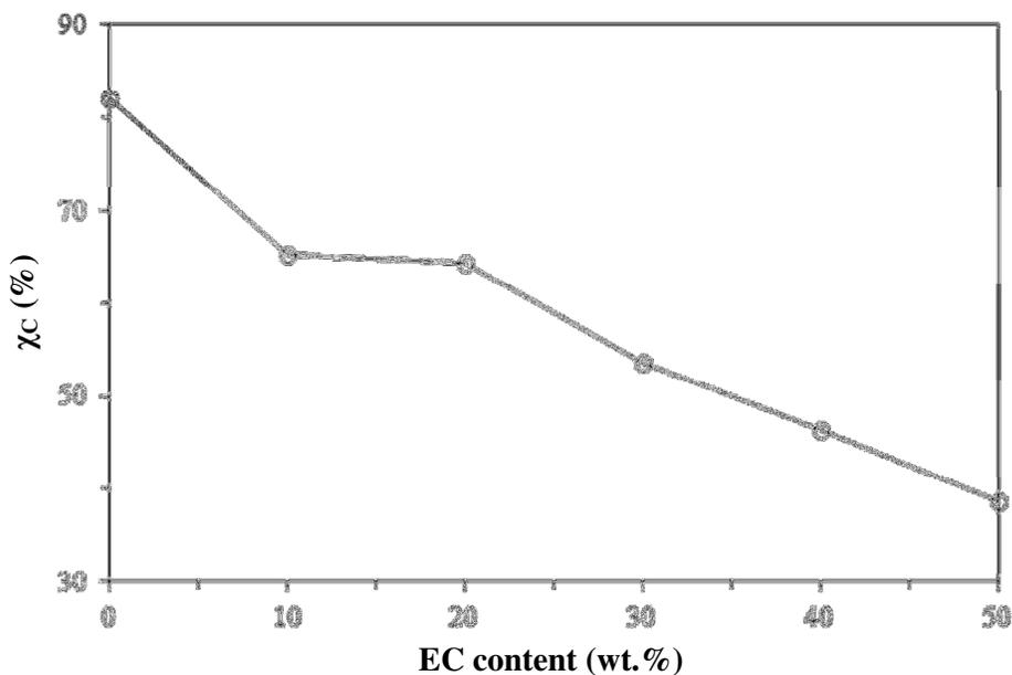
**Fig. 4.7** Relative degree of crystallinity as a function of EC content for PCL-NH<sub>4</sub>SCN-EC films added with 0 to 50 wt.% EC.
