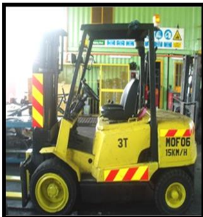
Figure 4.19 and 4.20: Improved forklift visibility
