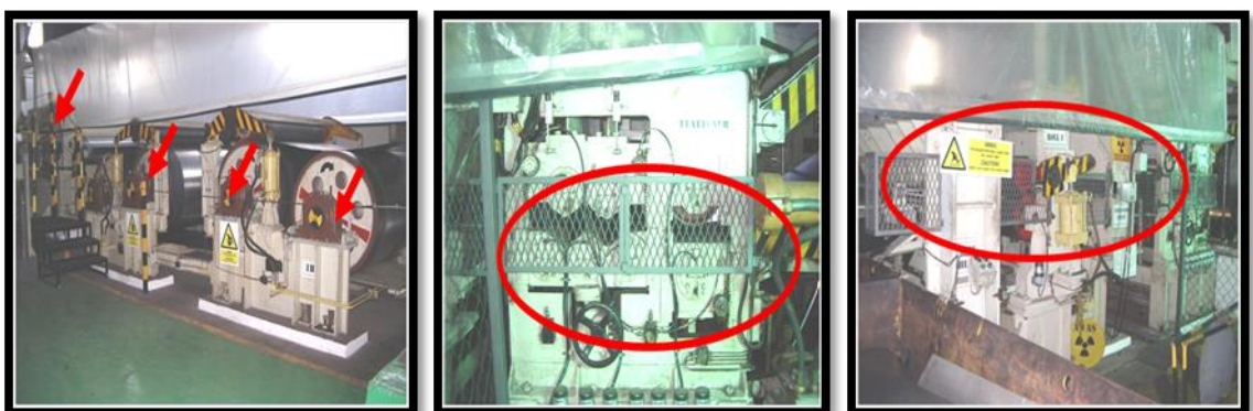
Figure 4.27: Safety Wire Trip
