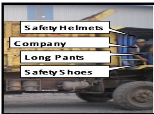
Figure 4.35: Driver Must Wear PPE Provided; safety helmet, long pants and safety shoes while driving and handling the vehicle
