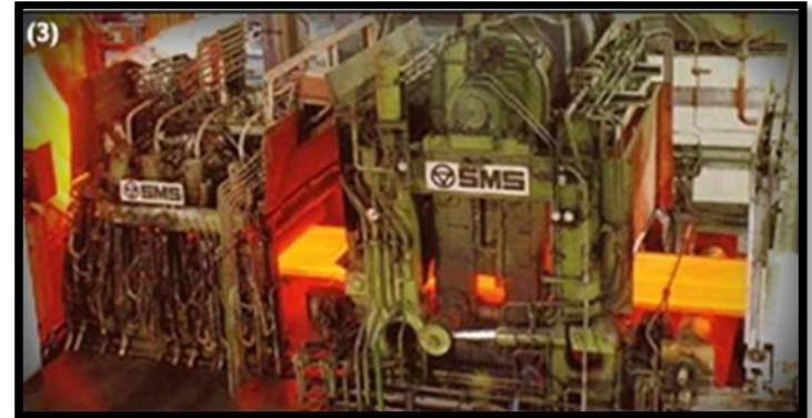
Fig.3.15: TSC Caster: To cast thin slabs
