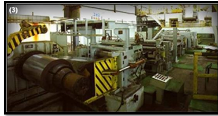
Fig 3.22: ECL: To clean and remove all emulsion stains from the strip before final coiling
