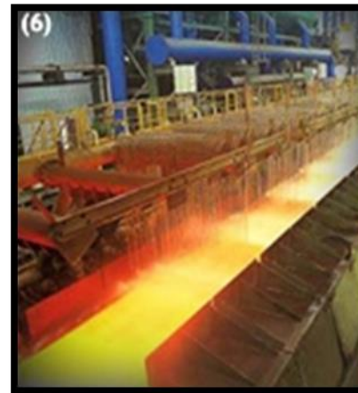
Fig. 3.18: LCS: To ensure coil's strip temperature & mechanical properties of surface quality
