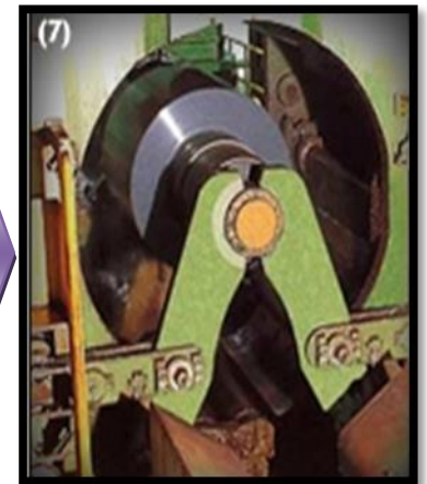
Fig.3.19: HSD: For coiling of strip into HRC
