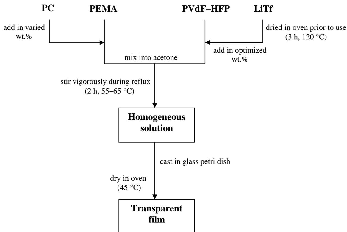
Figure 3.5 Flow chart for the preparation procedure of PEMA/PVdF-HFP-LiTf-PC polymer electrolyte films
