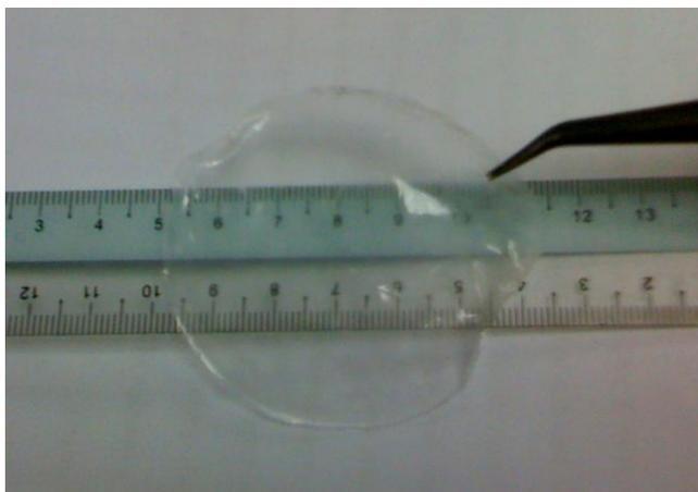
**Figure 3.3** Image of transparent PEMA/PVdF-HFP based polymer electrolytes
