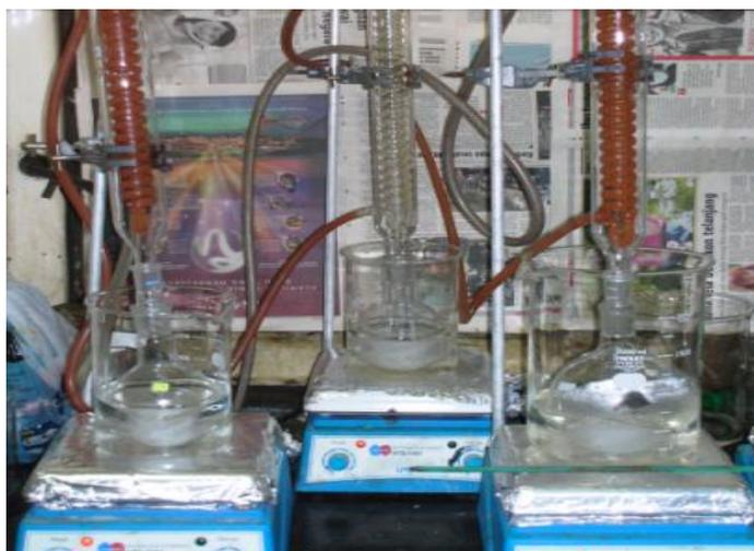
**Figure 3.1** Image of reflux set–up during preparation of polymer electrolytes
