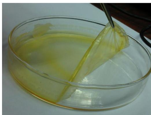
Figure 3.7 Image of semi-transparent PEMA/PVdF–HFP–LiTf–BMII based polymer electrolytes
