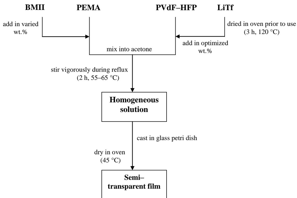
Figure 3.6 Flow chart for the preparation procedure PEMA/PVdF-HFP-LiTf-BMII polymer electrolyte films
