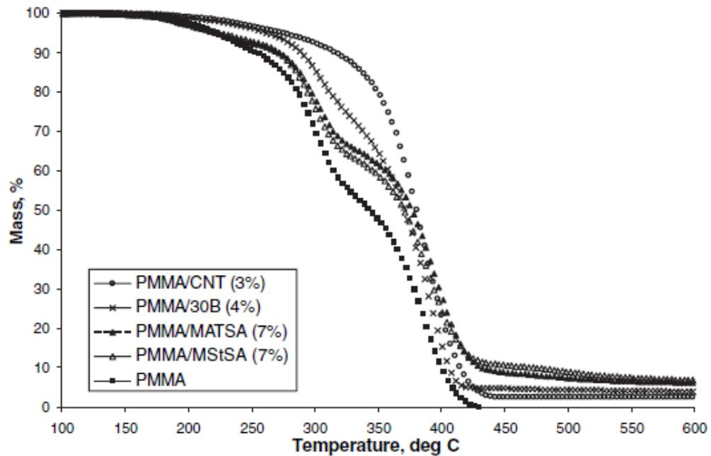
Figure 3.10 TGA curves of PMMA and its nanocomposites
