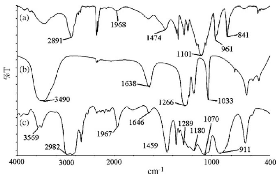
**Figure 3.9** FTIR spectra of (a) pure PEO, (b) pure LiTf and (c) PEO:LiTf (95:5; wt.:wt.) sample [Taken from Ramesh et al., 2008]
