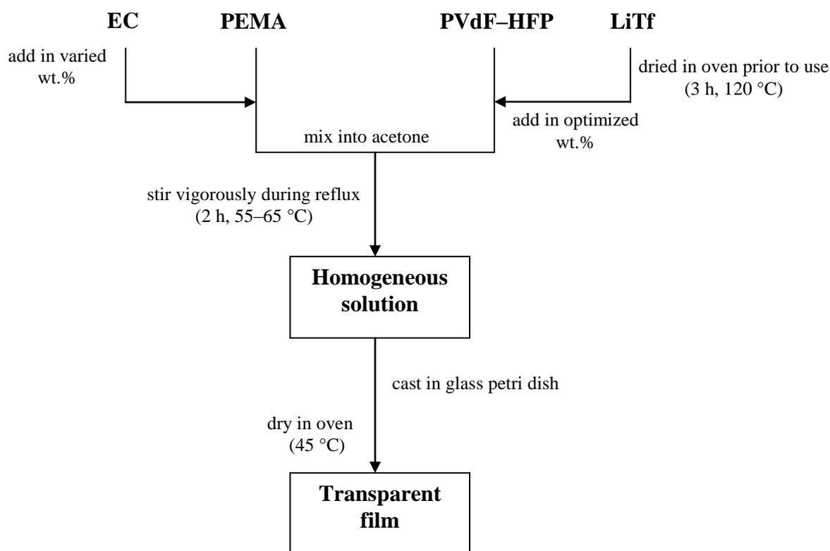
**Figure 3.4** Flow chart for the preparation procedure of PEMA/PVdF-HFP-LiTf-EC polymer electrolyte films
