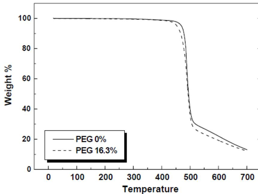
Figure 3.11 TGA thermograms of PVDF–HFP films containing 0 and 16.3 wt.% PEG
