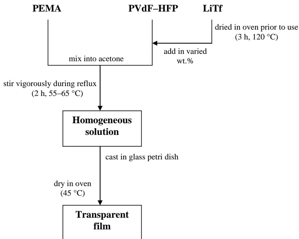
**Figure 3.2** Flow chart showing the preparation procedure of PEMA/PVdF-HFP-LiTf polymer electrolyte films
