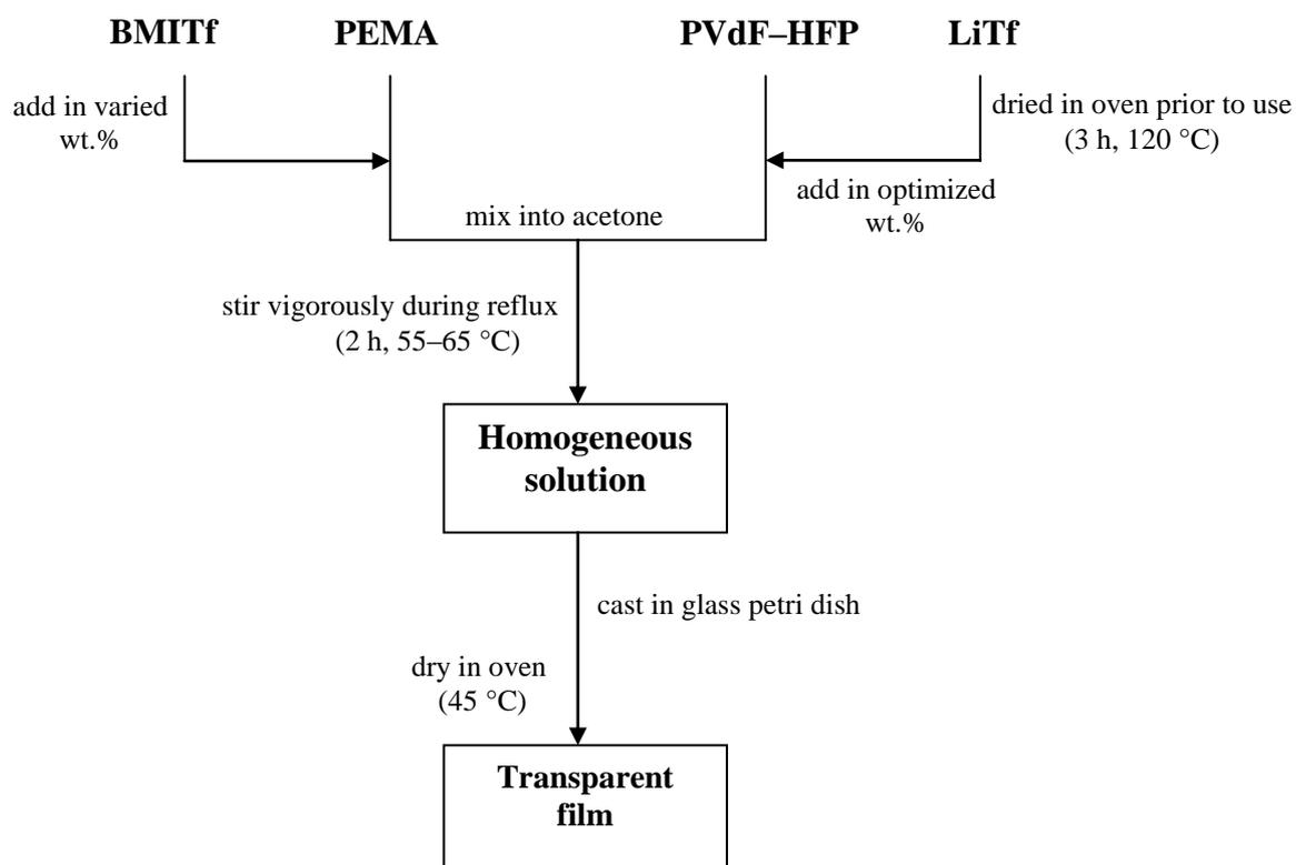
Figure 3.8 Flow chart for the preparation procedure of PEMA/PVdF–HFP–LiTf–BMITf polymer electrolyte films
