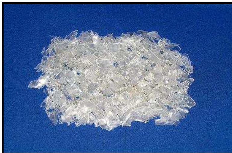
Figure A2-1 PET flakes from post-consumer PET bottles
