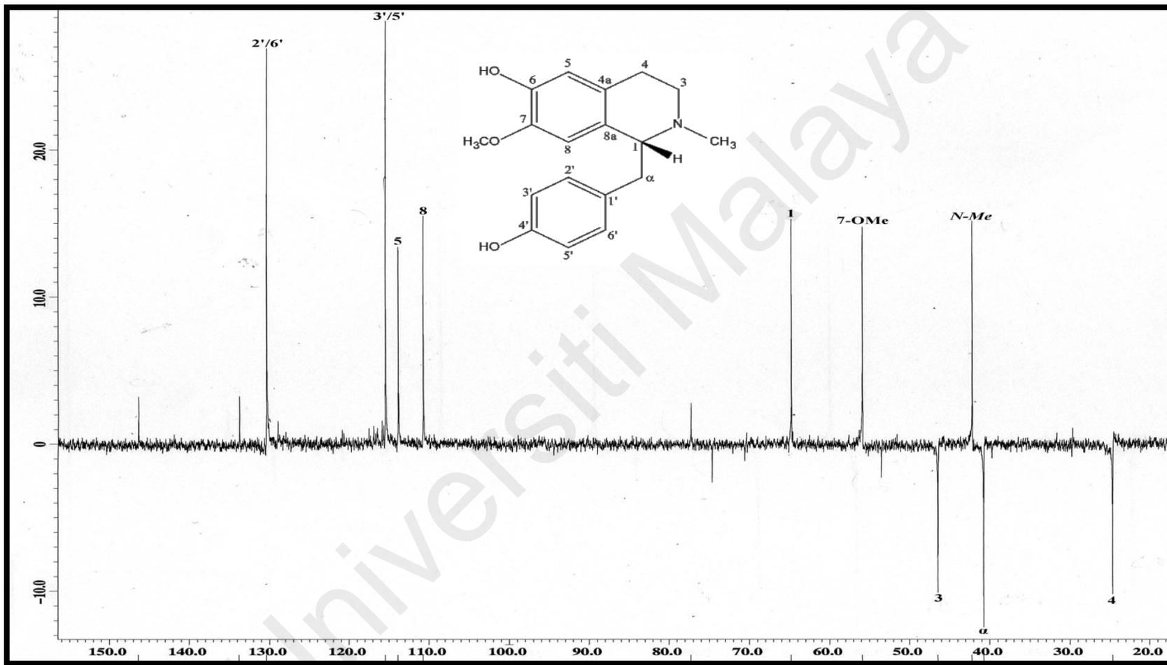
Figure 3.6: <sup>135</sup>DEPT NMR Spectrum of *N*-methylisococlaurine **46**
