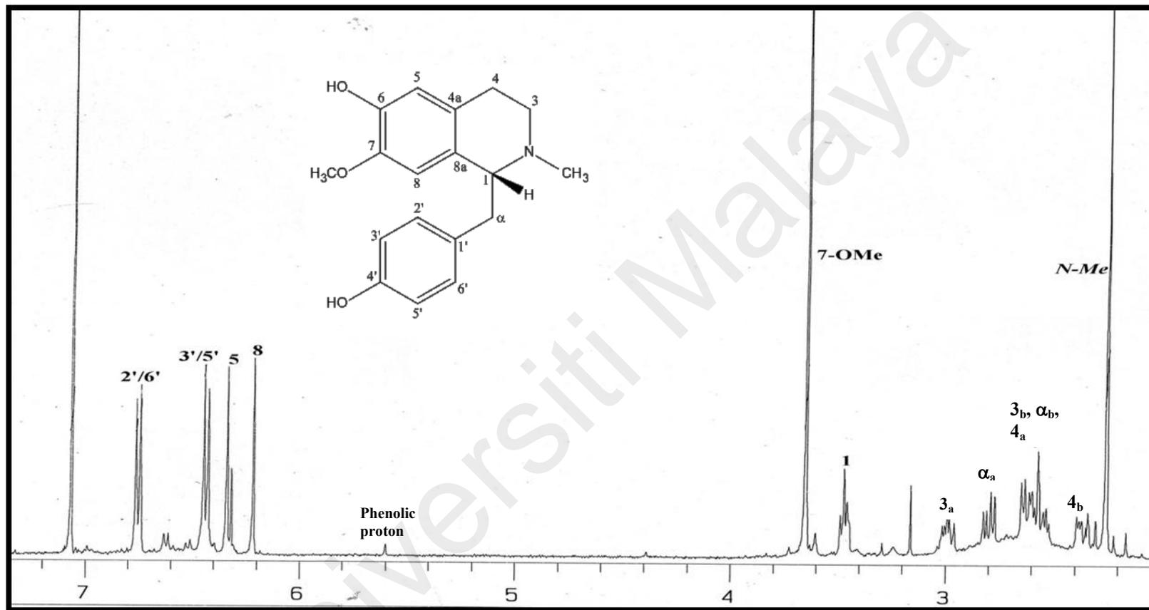
Figure 3.4:  $^1\text{H}$  NMR Spectrum of *N*-methylisococlaurine 46
