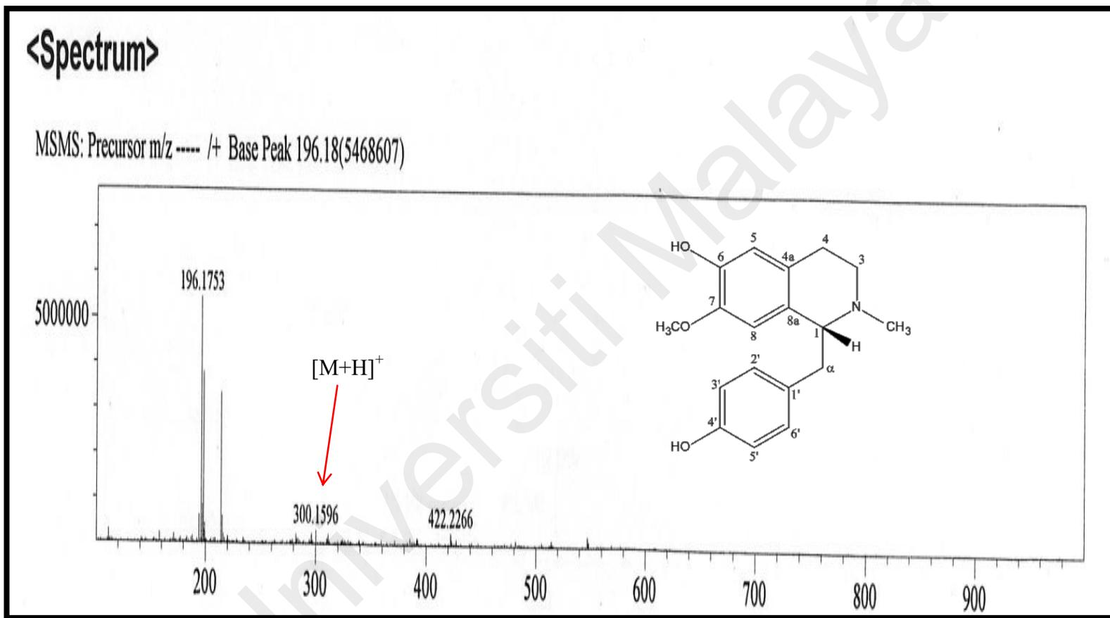
Figure 3.2: LCMS Spectrum of *N*-methylisococlaurine **46**
