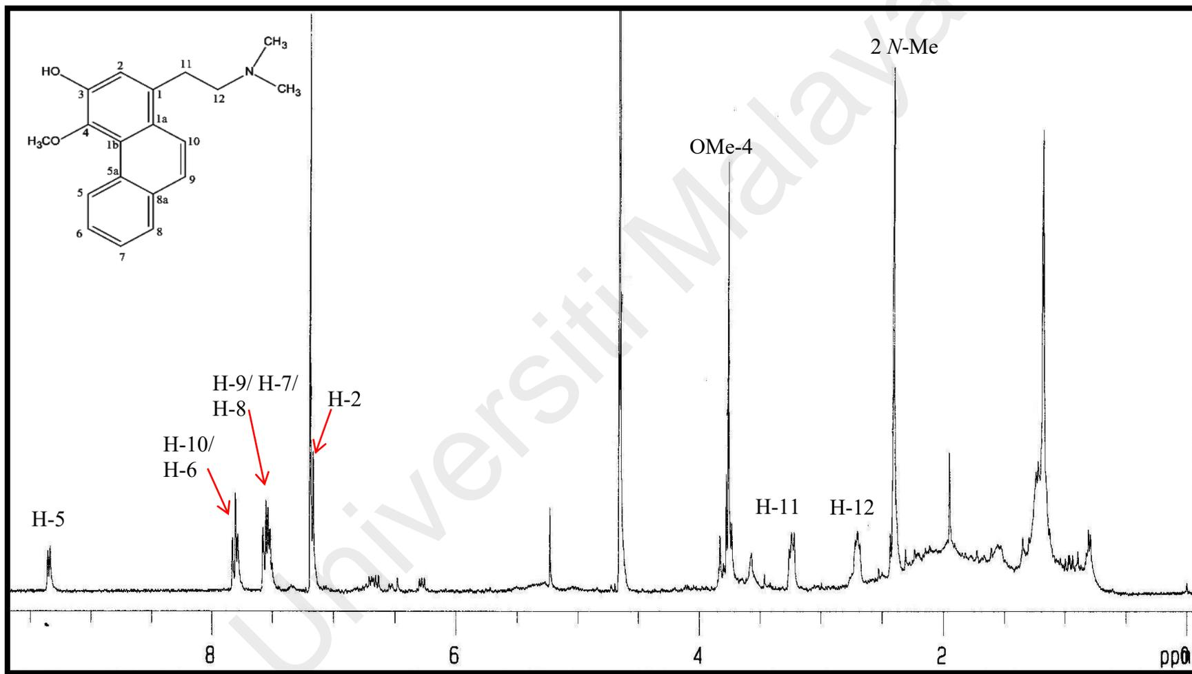
Figure 3.42: <sup>1</sup>H-NMR Spectrum of Argentinine 50
