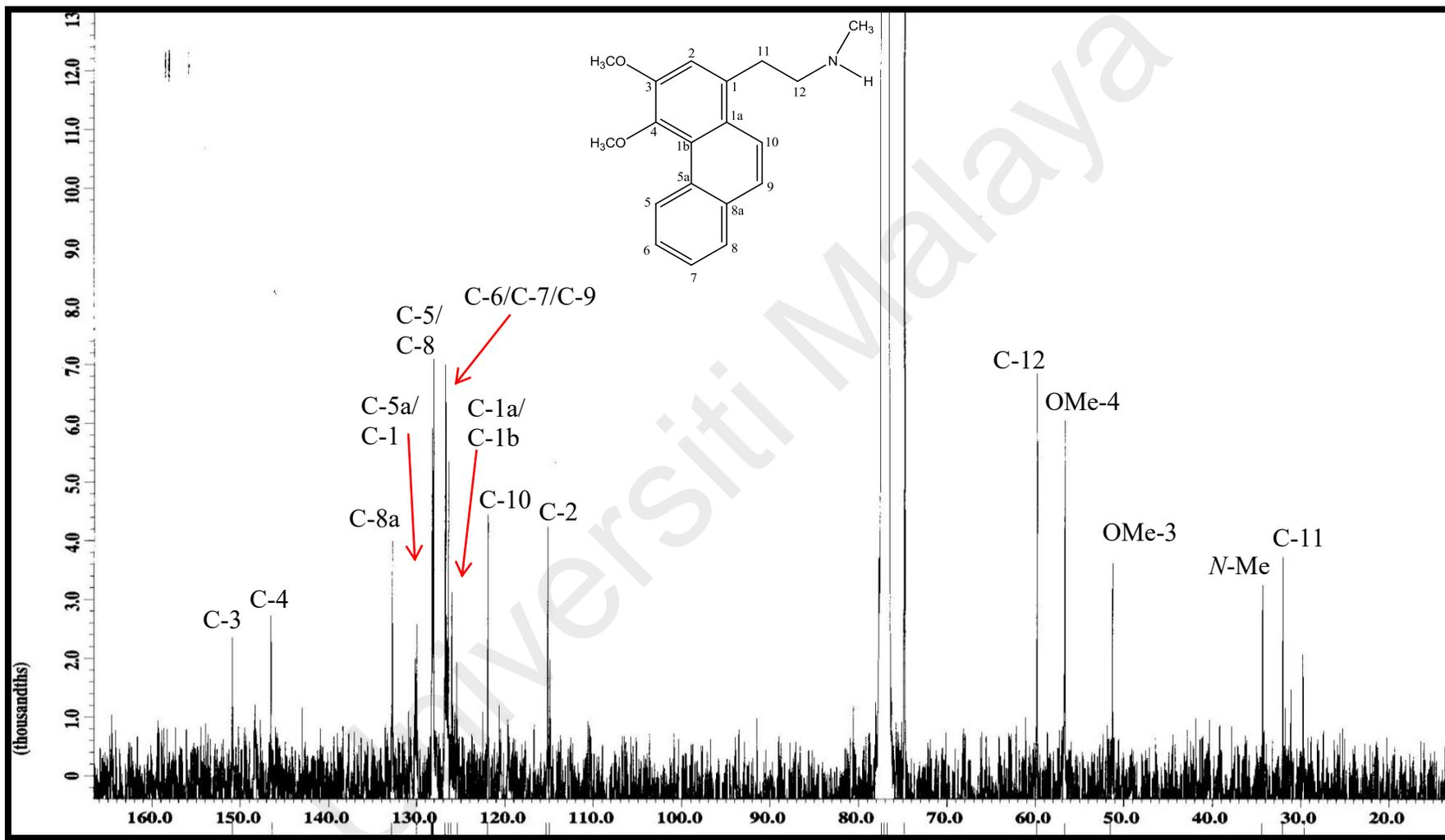
Figure 3.25:  $^{13}\text{C}$ -NMR Spectrum of Noratherosperminine 47
