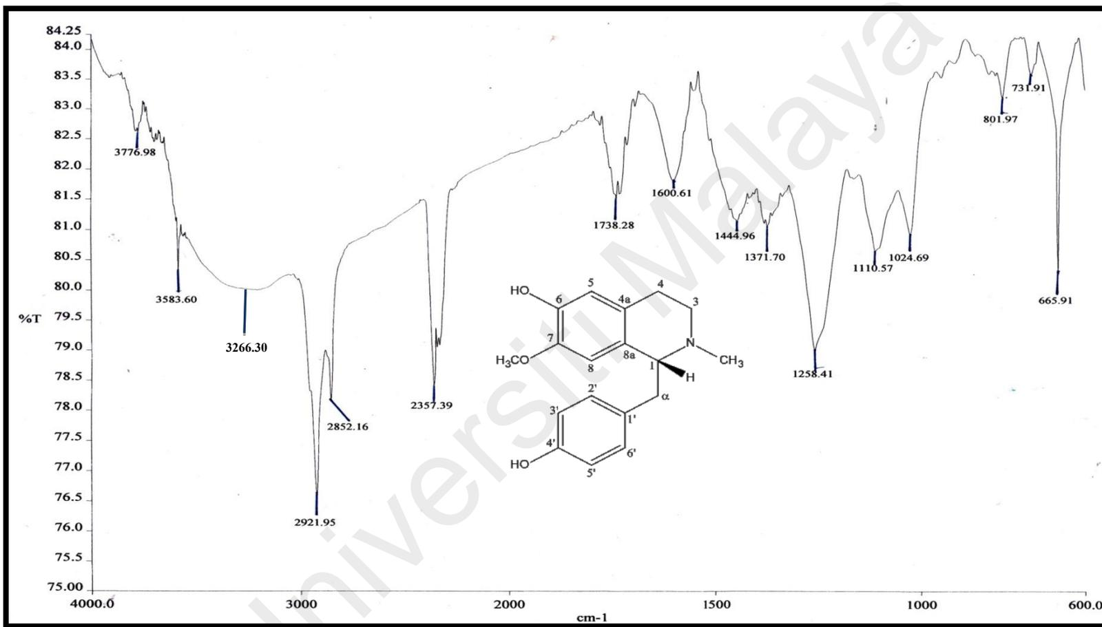
Figure 3.3: IR Spectrum of *N*-methylisococlaurine 46
