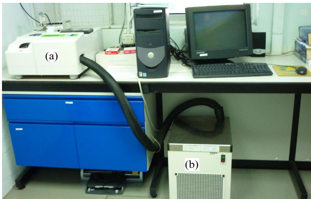
Figure 3.1: Mettler Toledo DSC (Model: DSC822e): (a) Temperature controller; (b) Intercooler
