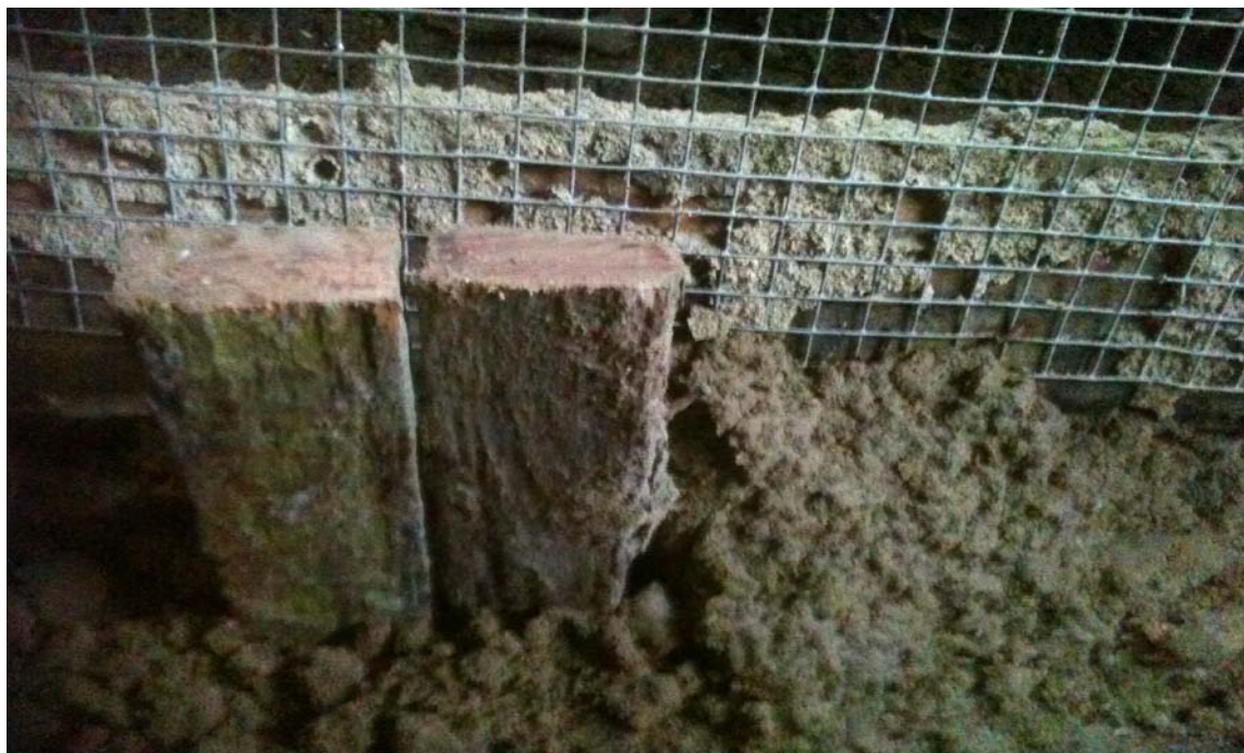
Plate 9. Treated and untreated blocks were inserted into termite infested area.
