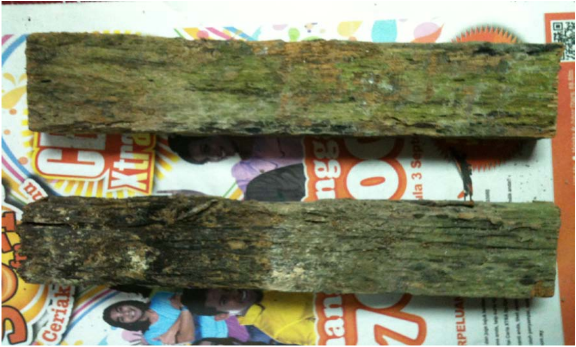
Plate 12. The blocks after 2 weeks of exposure to termite infested area.
