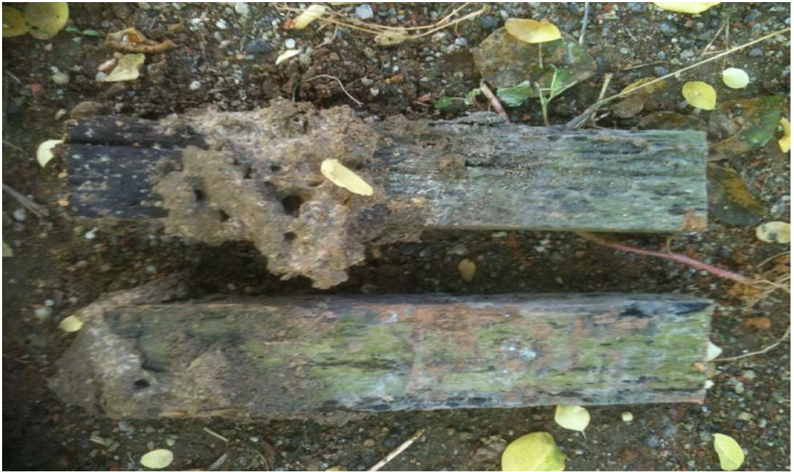
Plate 11. Treated and untreated blocks after 2 weeks of exposure to termite infested area.
