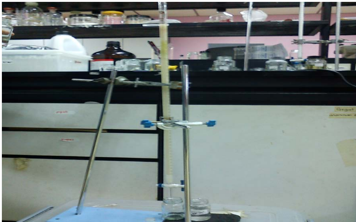
Plate 7. Separation of crude extract by column chromatography
