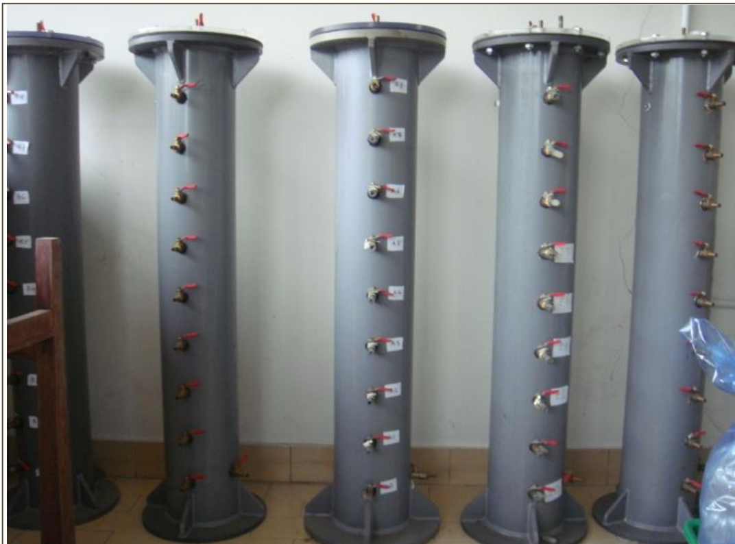
Plate 3.13: The PVC columns used for both laboratory and landfill experiment
