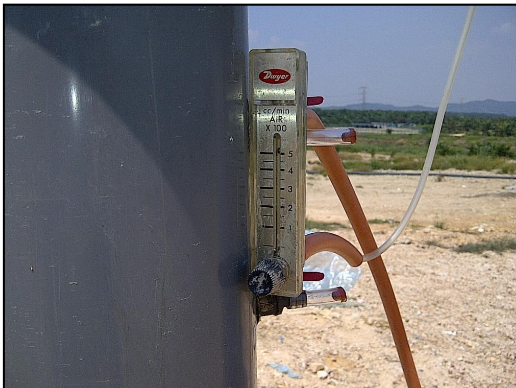
Plate 3.15: The Dwyer Rate Master flow meter is adjusted according to the amount of CH 4 and O 2 supply needed
