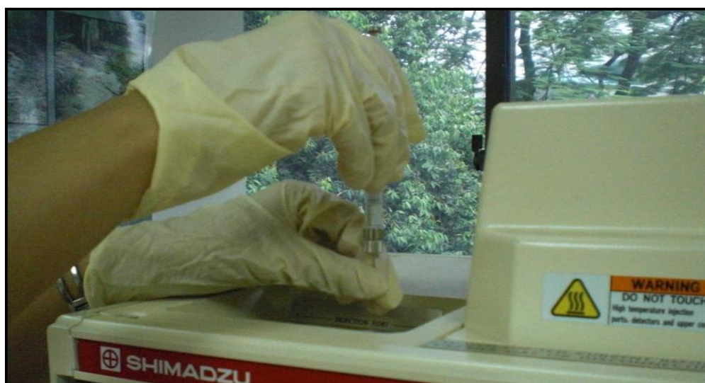
Plate 3.12: Injection of gas sample to GC
