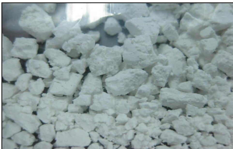
Figure 3.3: Polyethylene obtained from the polymerization using CI[1] and Al/Cr molar ratio of 26.2 at 30°C
